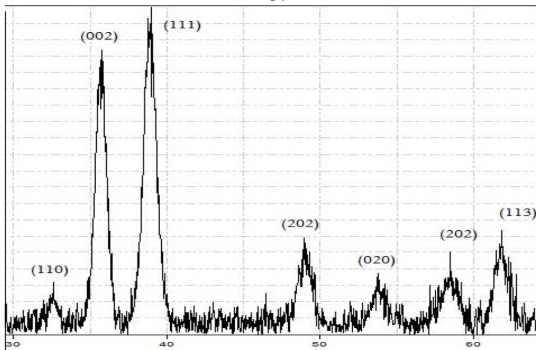
**Fig 3.5: XRD pattern of CuO nanoparticles were prepared at 85 °C with TOAB surfactant**
