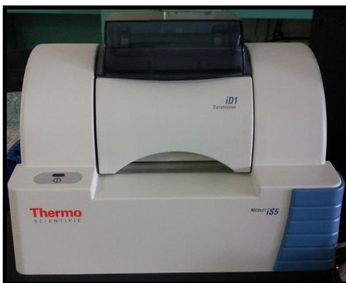
**Figure 3.1:** Fourier Transform Infra-Red spectroscopy.
