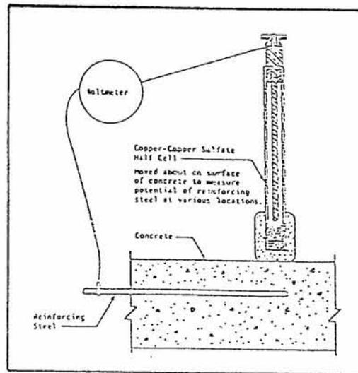
Figure 7. Half-Cell Potential Measurement Set-up (ASTM C 876).
