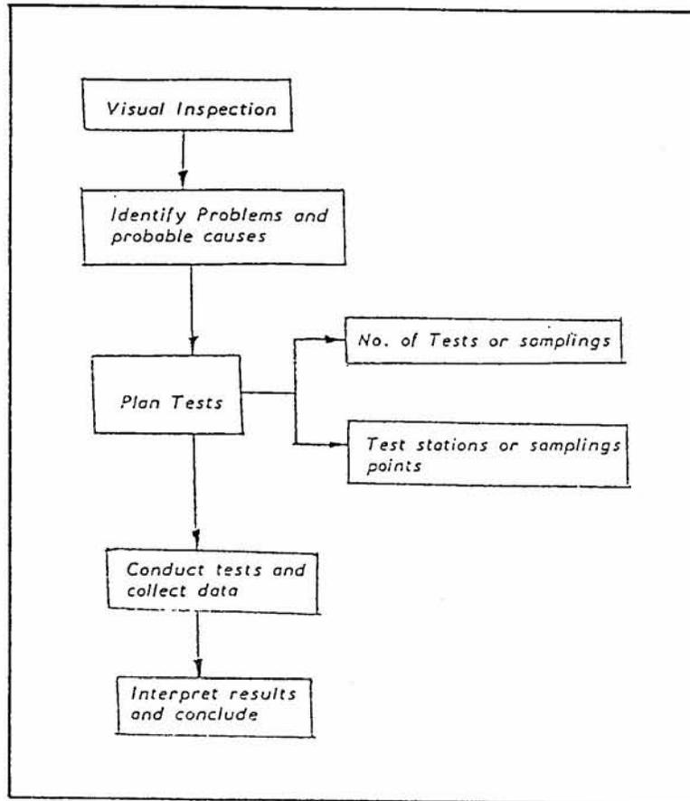
Figure 1. Flow chart of an in-situ test program.
