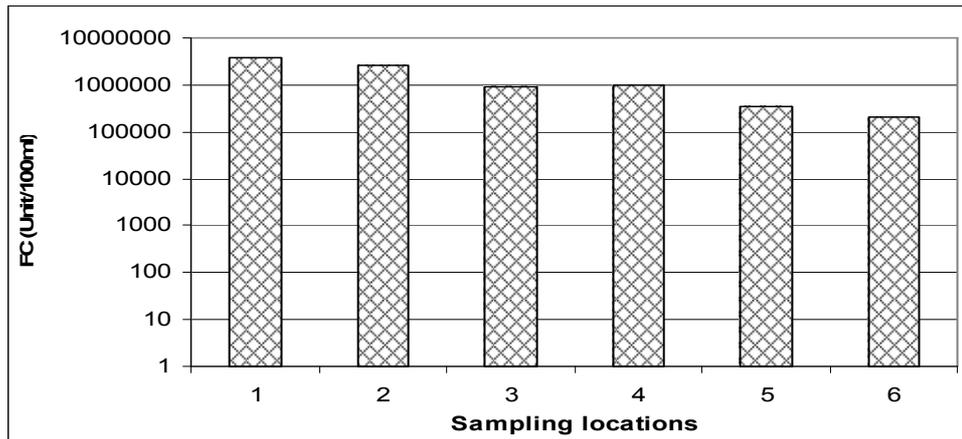
**Figure 10:** Average FC count of the different sampling locations of the treatment plant.
