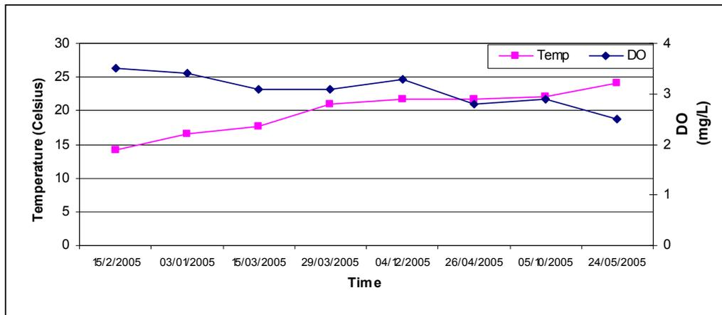
**Figure 2:** Average dissolved oxygen and temperature values over the time in location 4.
