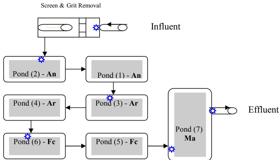
**Figure 1:** Flow diagram of treatment system and sampling points.
