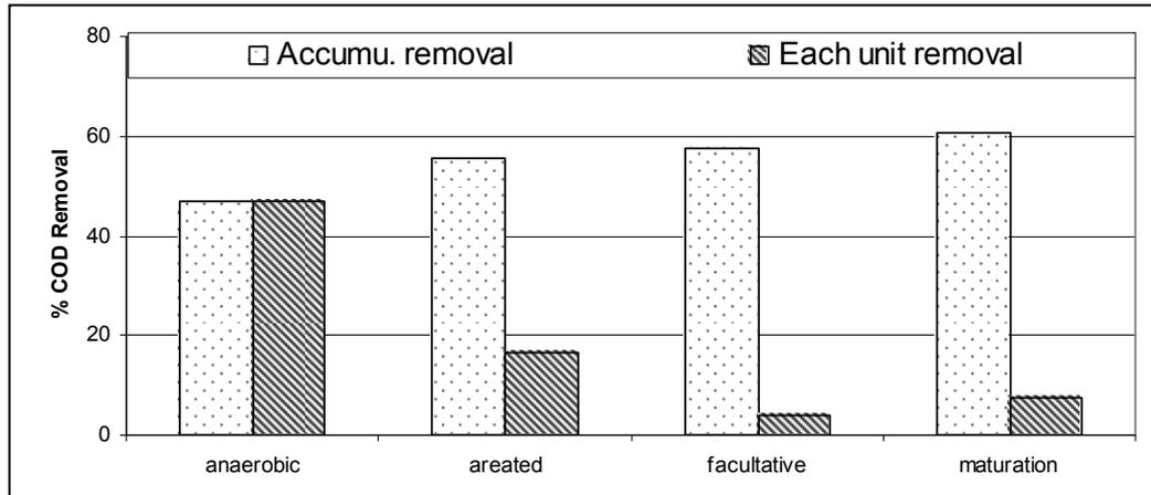
**Figure 7:** COD average percentage removal efficiency and accumulative removal effects of different ponds types.
