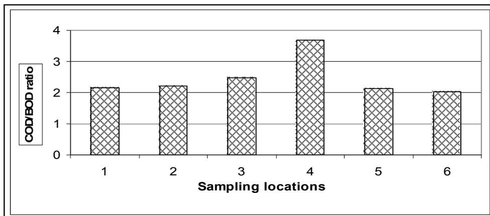
**Figure 8:** Average COD: BOD<sub>5</sub> ratio at different sampling points.
