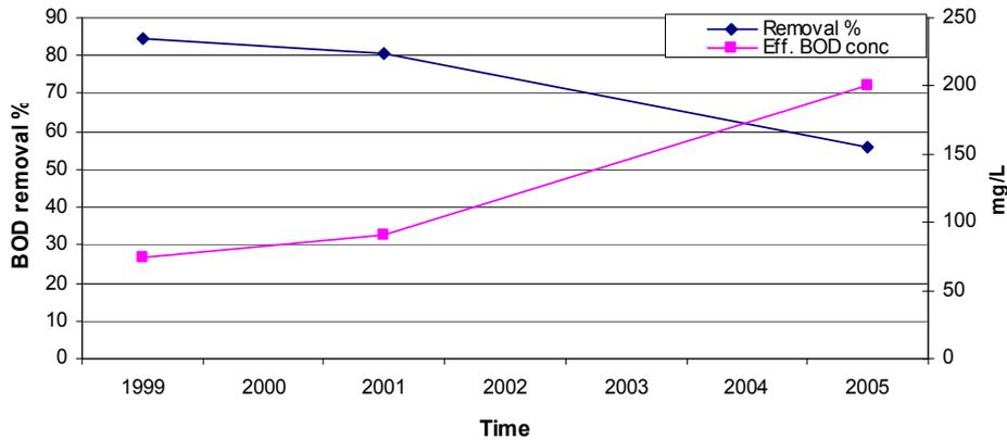
**Figure 6:** Percentage removal and effluent concentration of BOD<sub>5</sub>.
