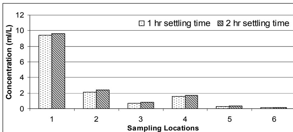
**Figure 4:** Average settleable solids after one and two hour concentration at different sampling points.
