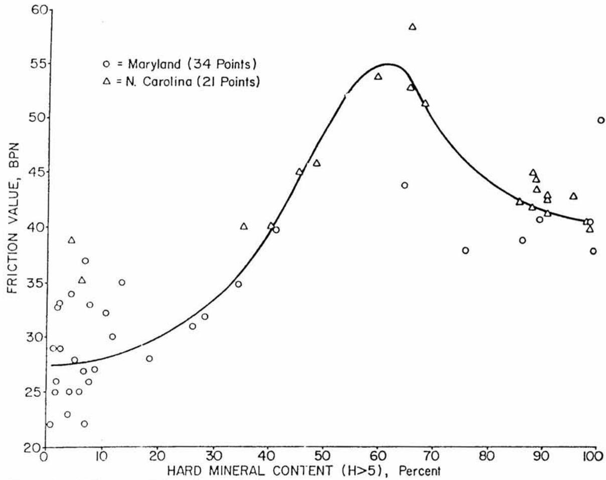
Figure 4. BPN Friction Values (ASTM E 303) Versus Hard Mineral Content [8].
