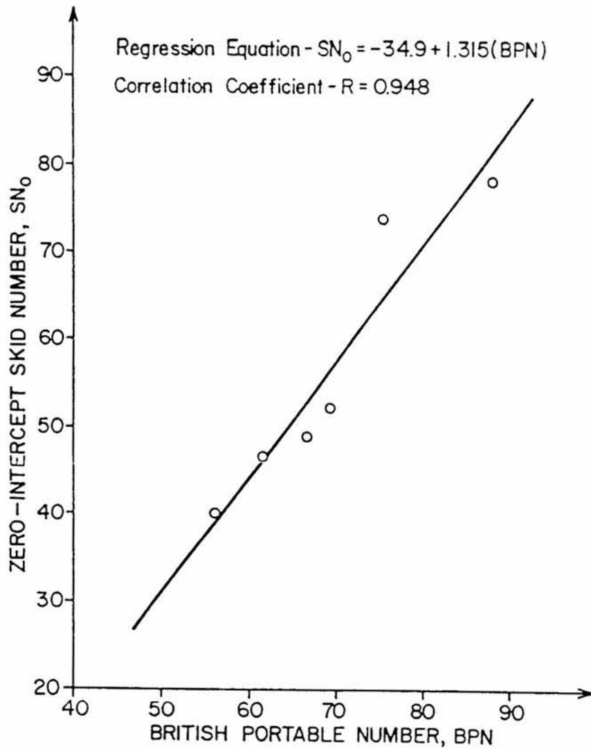
Figure 6. Zero-Intercept Skid Number vs. British Portable Number [6]
