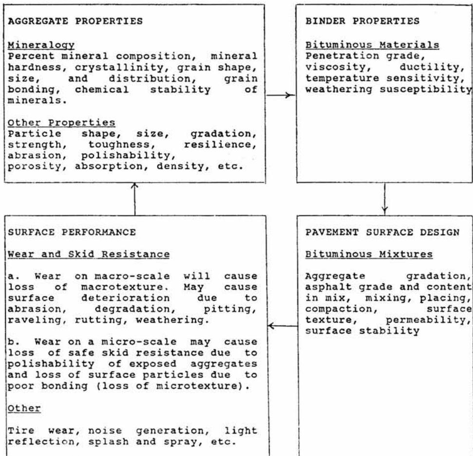
Figure 2: Relationships between Surface Materials and/or Design and Surface Performance
