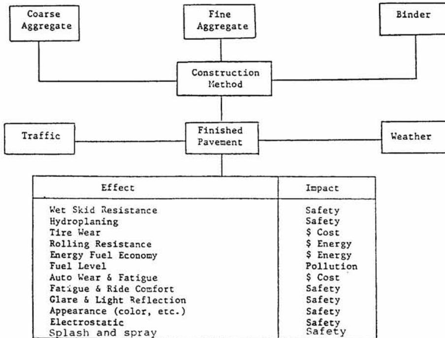
Figure 1. Role of Aggregates on Surface Properties and the Subsequent Penalties and Benefits of the Surface Properties
