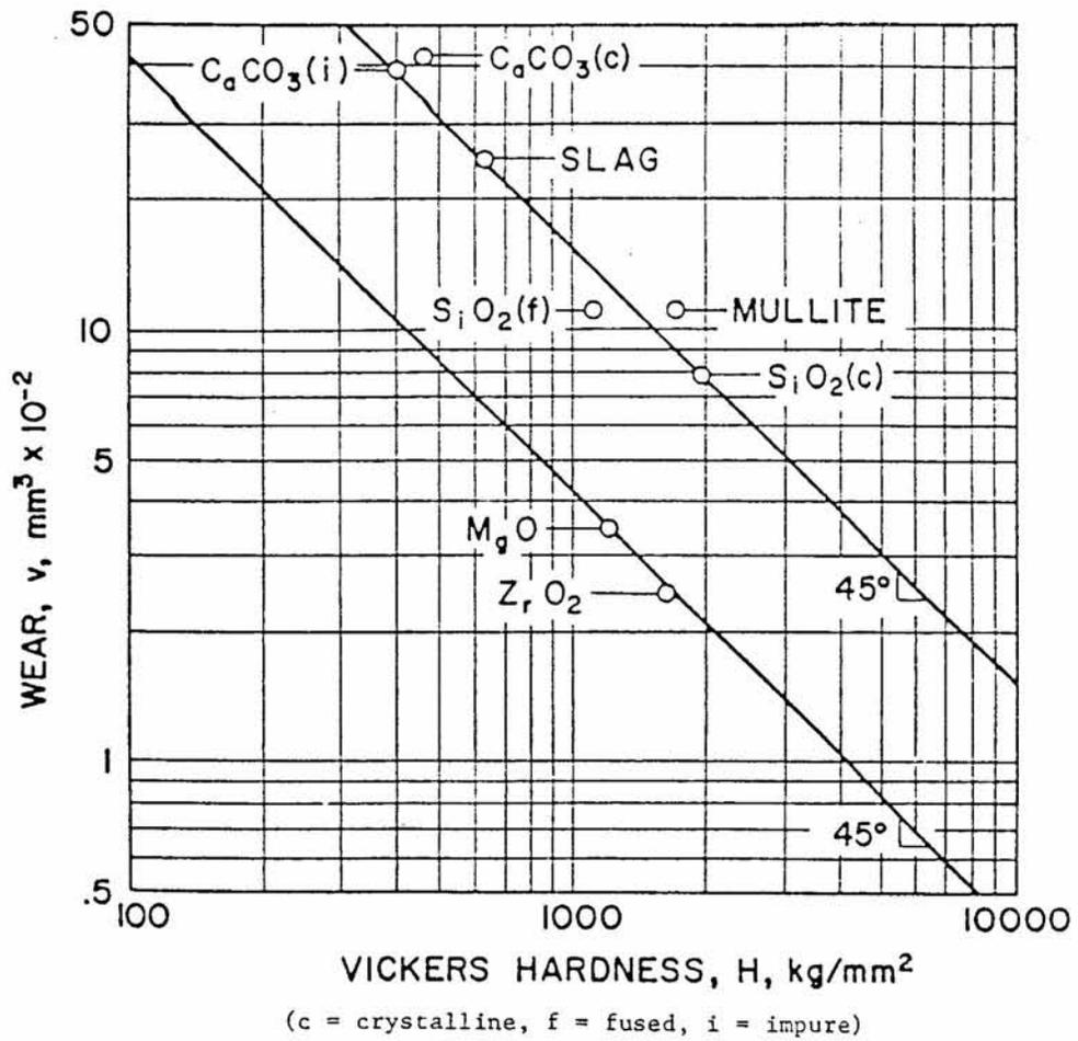
Figure 3. Log Wear as a Function of Log Hardness for Minerals Softer than  $\text{Al}_2\text{O}_3$  Abrasive [1]
