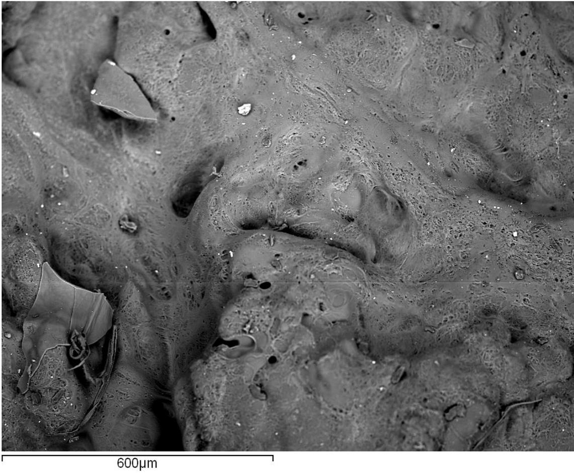
**Fig. a5:** Electronic Image for prepared SAP (PAA-AS), Input Source: Secondary electron detector, Image Width: 1.263 mm
