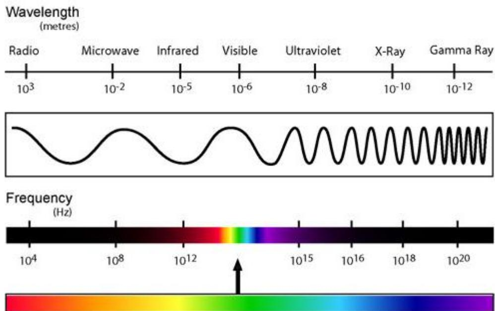
**Fig. (1.1):** The Electromagnetic Spectrum.
