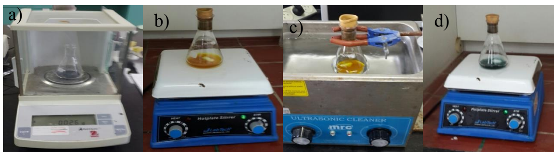
Fig. (3.1): Steps of preparing sol-gel solution: (a) weighting, (b) stirring, (c) sonificating, (d) the color change of the solution from yellow to blue.
