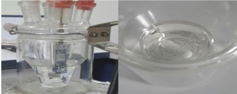
Fig. (4.6): W_{0.95}Ti_{0.05}O_3 film degradation after 6000 th cycles.
