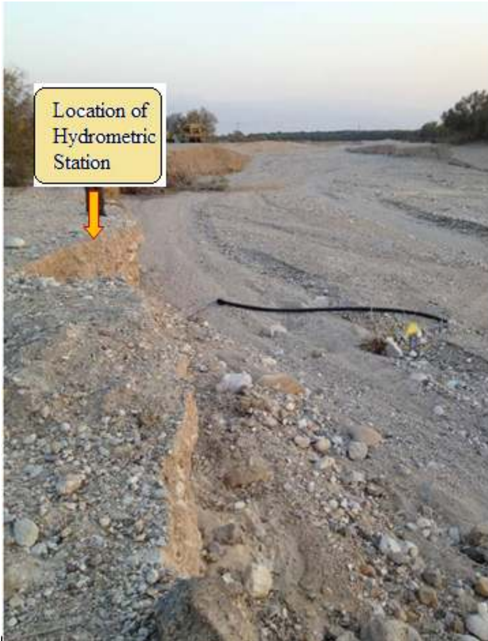
Figure (6-4): Location of the Draggged Hydrometric Station and the Remains of the Pipe after 8th January flood at Og Watershed
