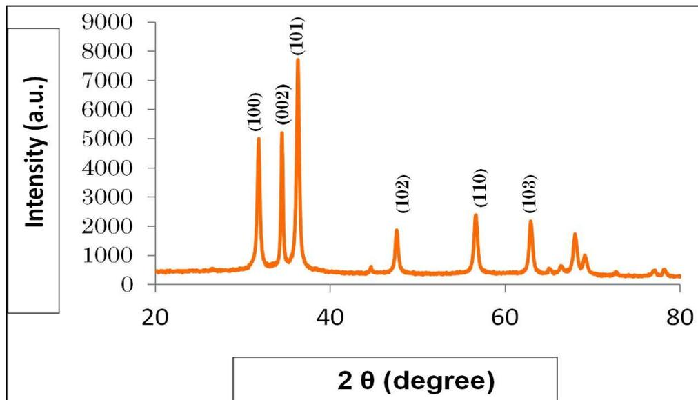
**Figure (3.2):** X-ray diffraction patterns of nano size zinc oxide ( ZnO) particles [63].
