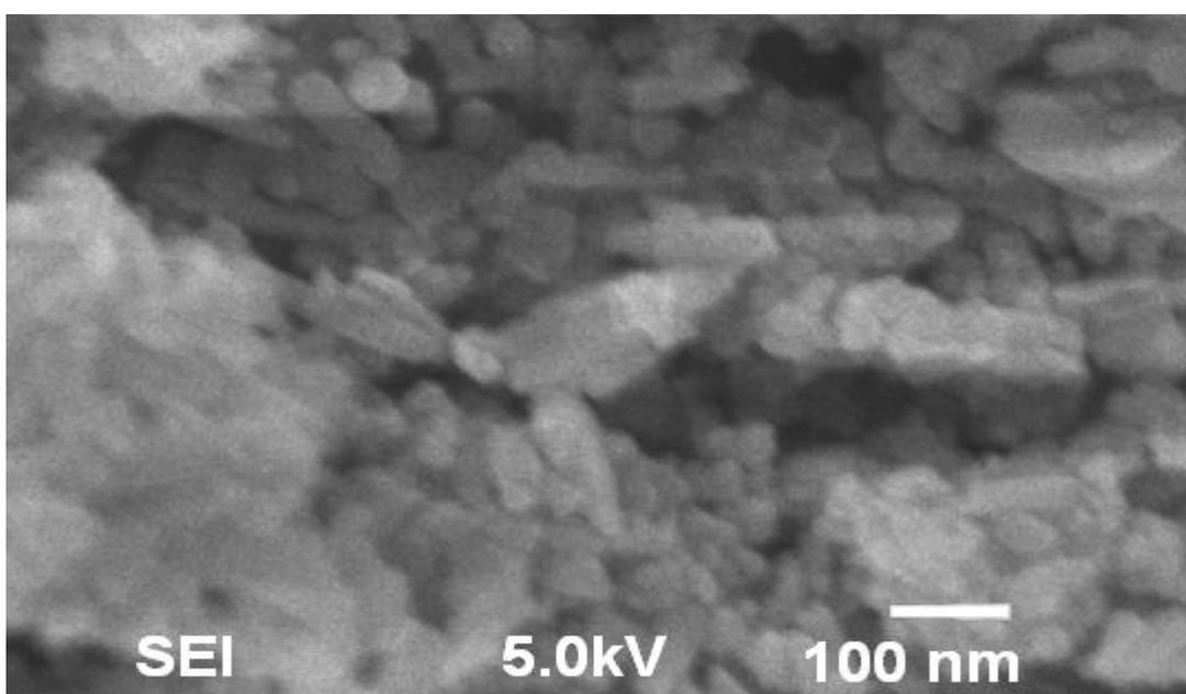
**Figure (3.3):** SEM images for the prepared ZnO nanoparticles [63].
