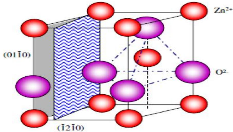
**Figure (1.1):** Wurtzite structure of ZnO [42]
