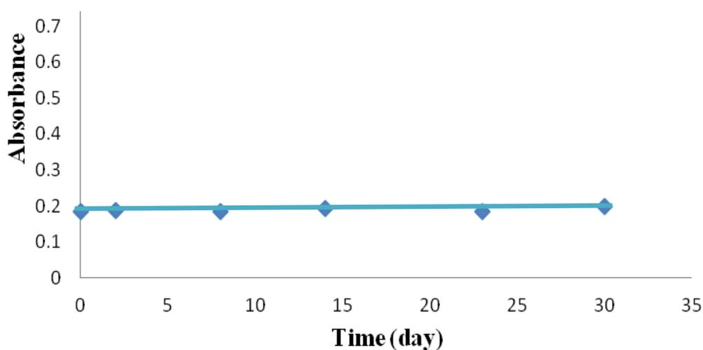
**Figure 3.26:** Effect of time on Cu(II)–TAHA complex stability,  $[\text{Cu}^{2+}] = [\text{TAHA}] = 3 \times 10^{-3} \text{ M}$ , at pH 10,  $\lambda = 736 \text{ nm}$ .
