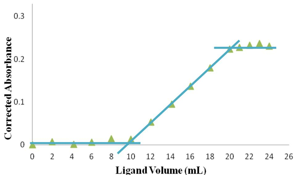
**Figure 3.14:** Spectrophotometric titration curve for the titration of  $\text{Cu}^{2+}$ -  $\text{Ca}^{2+}$  mixture (10 mL of 0.01 M each) with a 0.01 M TAHA. (pH = 10,  $\lambda = 736$  nm). Absorbance was corrected by the modified correction method.
