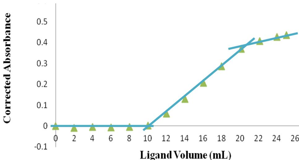
**Figure 3.19:** Spectrophotometric titration curve for the titration of  $\text{Cu}^{2+}$ -  $\text{Co}^{2+}$  mixture (10 mL of 0.01 M each) with a 0.01 M TAHA. ( $\text{pH} = 10$ ,  $\lambda = 736$  nm). Absorbance was corrected by the modified correction method.
