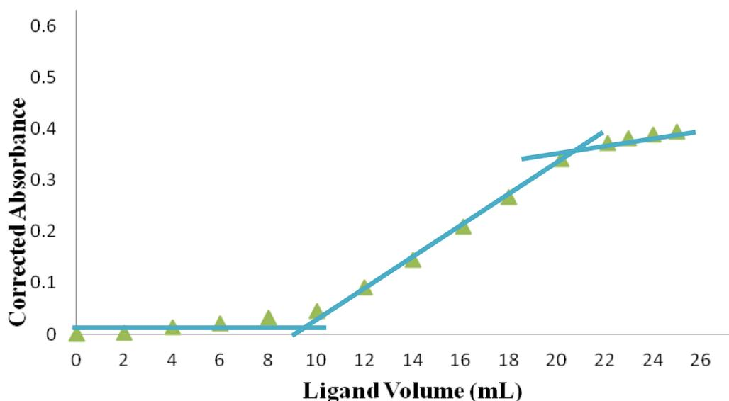
**Figure 3.24:** Spectrophotometric titration curve for the titration of  $\text{Cu}^{2+}$ -  $\text{Cd}^{2+}$  mixture (10 mL of 0.01 M each) with a 0.01 M TAHA. (pH = 10,  $\lambda = 736$  nm). Absorbance was corrected by the modified correction method.
