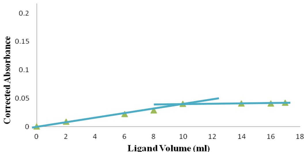
**Figure 3.12:** Spectrophotometric titration curve for the titration of 10 mL of 0.01 M  $\text{Ni}^{2+}$  with a 0.01 M TAHA. ( $\text{pH} = 10$ ,  $\lambda = 557 \text{ nm}$ ). Absorbance was corrected by the modified correction method.
