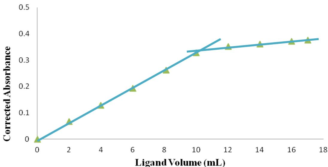
**Figure 3.8:** Spectrophotometric titration curve for the titration of 10 mL of 0.01 M  $\text{Cu}^{2+}$  with 0.01 M TAHA. ( pH = 10,  $\lambda = 736$  nm). Absorbance was corrected by the modified correction method.
