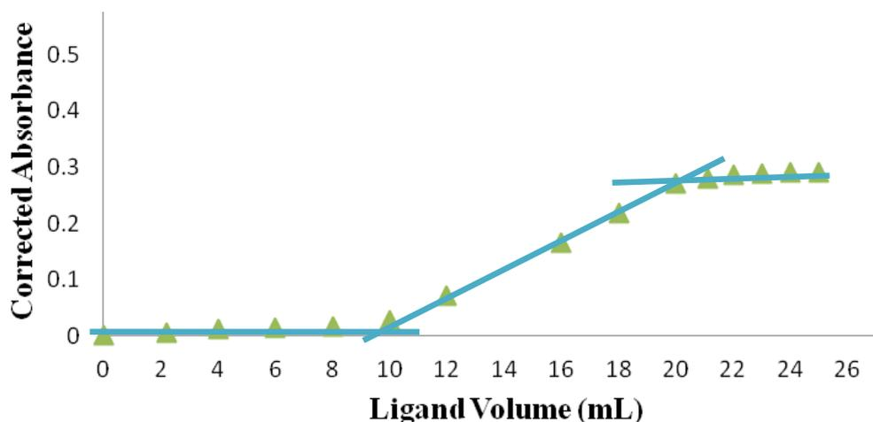
**Figure 3.22:** Spectrophotometric titration curve for the titration of  $\text{Cu}^{2+}$ - $\text{Ni}^{2+}$  mixture (10 mL of 0.01 M each) with a 0.01 M TAHA. ( $\text{pH} = 10$ ,  $\lambda = 736$  nm). Absorbance was corrected by the modified correction method.
