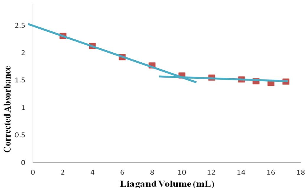
**Figure 3.9:** Spectrophotometric titration curve for the titration of 10 mL of 0.01 M  $\text{Co}^{2+}$  with a 0.01 M TAHA. (pH = 10,  $\lambda = 309$  nm). Absorbance was corrected for dilution.
