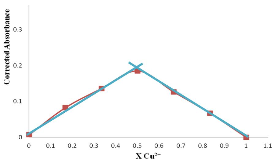
**Figure 3.25:** Curve for the continuous variation method, for Cu(II)–TAHA Complex at pH 10,  $\lambda = 736 \text{ nm}$ .
