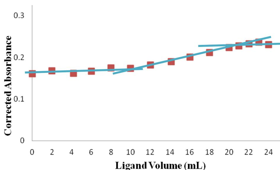
**Figure 3.13:** Spectrophotometric titration of  $\text{Cu}^{2+}$ -  $\text{Ca}^{2+}$  mixture (10 mL of 0.01 M each) with 0.01 M TAHA. (pH = 10,  $\lambda$  = 736 nm). Absorbance was corrected for dilution.
