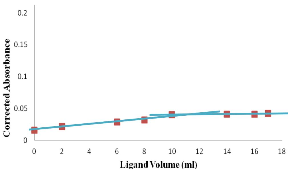
**Figure 3.11:** Spectrophotometric titration curve for the titration of 10 mL of 0.01M Ni<sup>2+</sup> with a 0.01M TAHA. (pH = 10,  $\lambda = 557$  nm). Absorbance was corrected for dilution.
