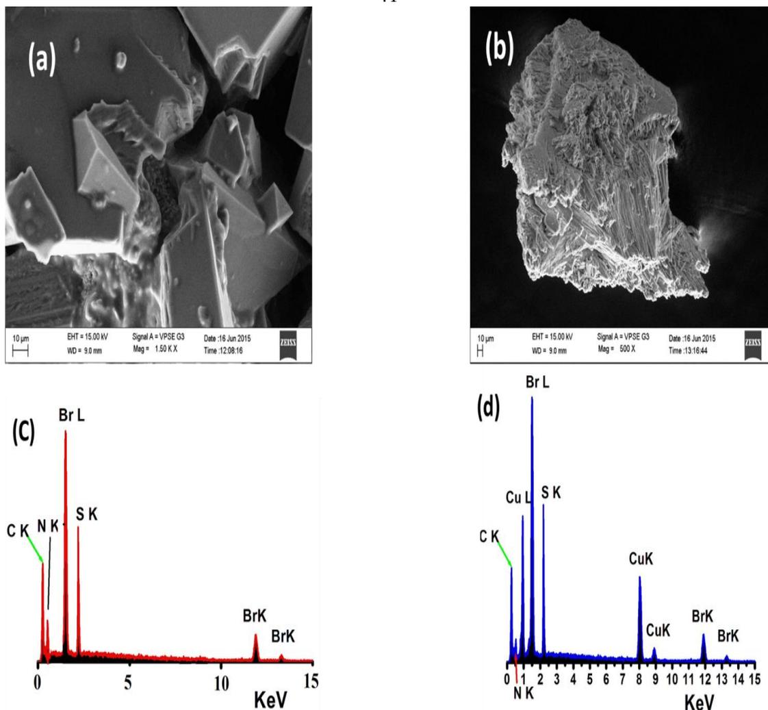
**Fig. (3.13):** SEM Images of (a) N<sub>3</sub>S<sub>2</sub> Ligand, (b) Complex 2, and EDS Images of (c) N<sub>3</sub>S<sub>2</sub> Ligand; (d) Complex 2.
