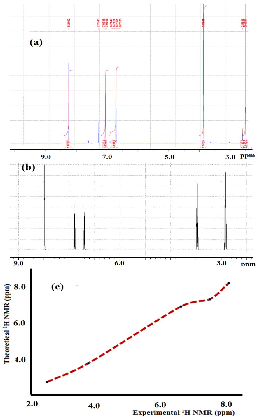
**Fig. (3.3):**  $^1\text{H}$  NMR Spectra of Desired Ligand (a) Experimentally in  $\text{CDCl}_3$  at RT, (b) Theoretically (c) Experimentally in Comparison to The theoretically Obtained.
