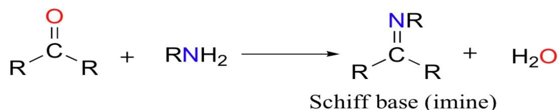
**Scheme 1:** General Procedure of Synthesis of Schiff Base.
