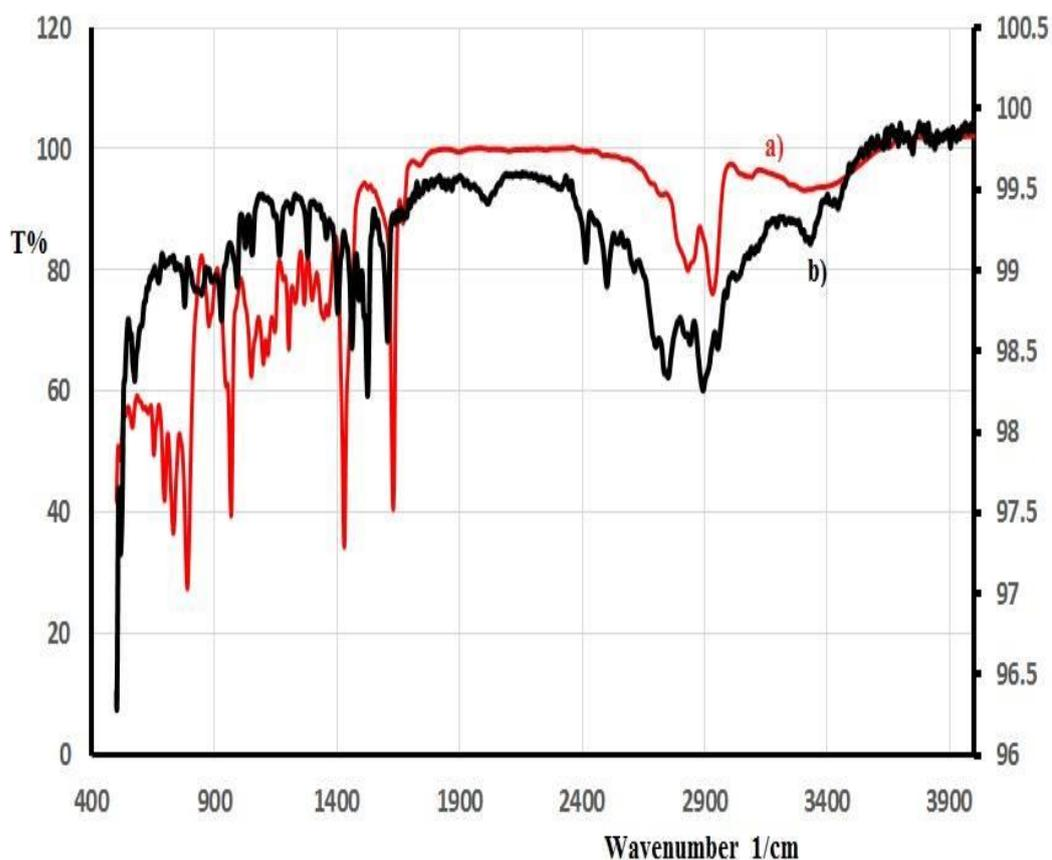
**Fig. (3.18):** IR-KBr Disk Spectra of a) Free **L2** and b) Complex **4** (with  $\text{CuBr}_2$ ).
