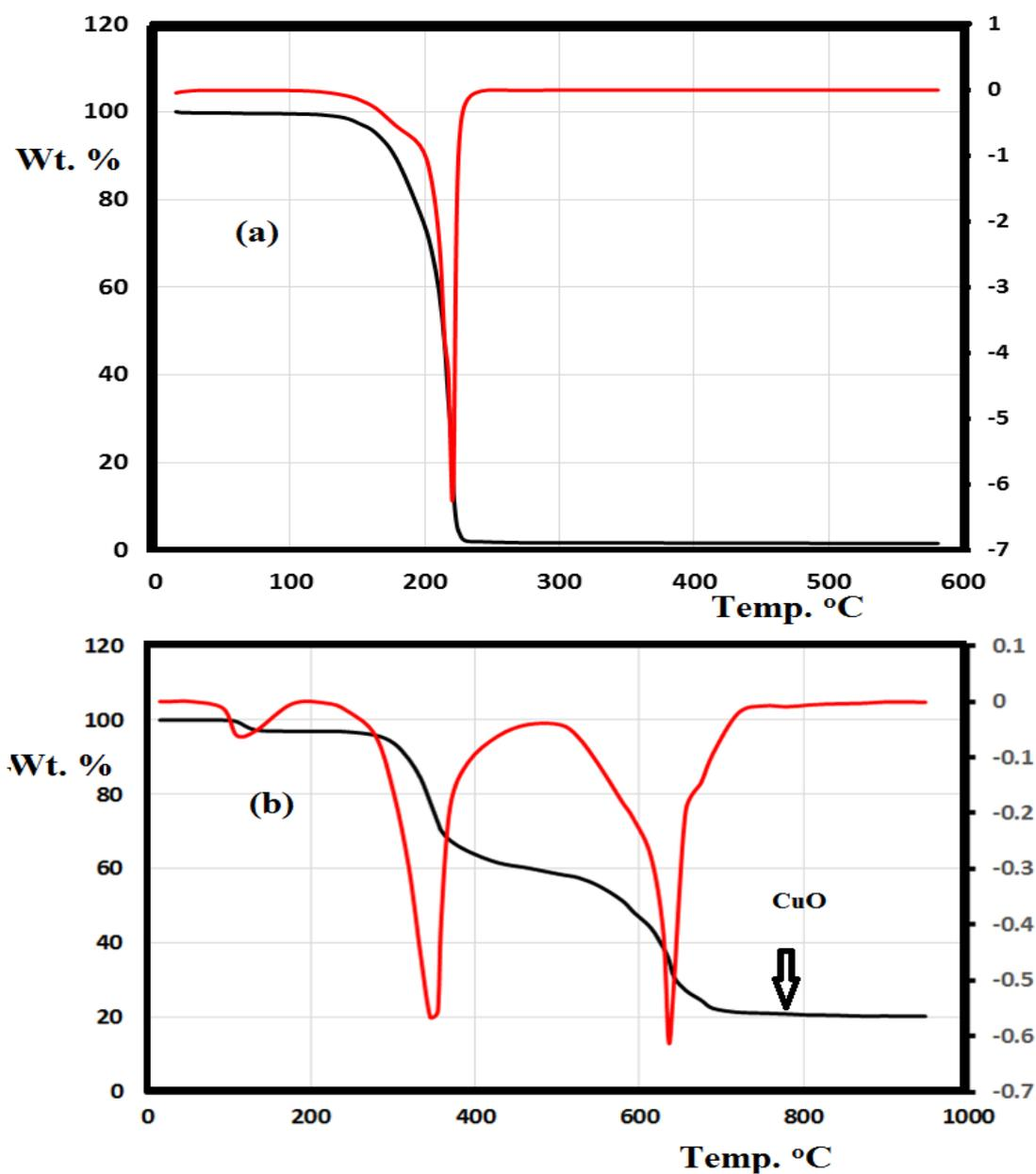
**Fig. (3.11):** TG/DTG Thermal Curves of: (a) the Ligand and (b) its Complex 2.
