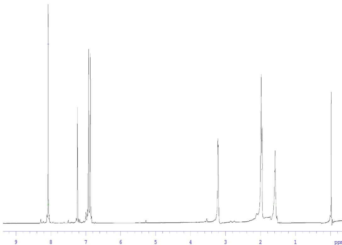
**Fig. (3.14):** Experimental  $^1\text{H}$  NMR (ppm) Spectrum of Desired **L2** Ligand Dissolved in  $\text{CDCl}_3$  at RT.
