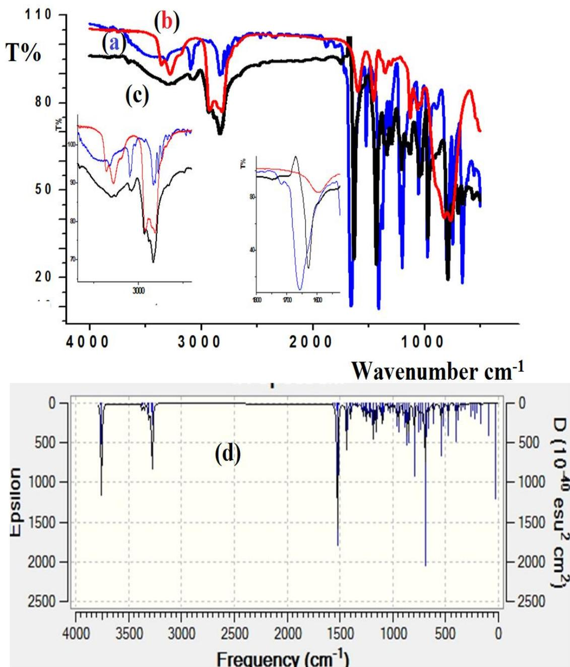
**Fig. (3.5):** IR Spectra of: (a) 5-Bromothiophene-2-Carbaldehyde, (b) Diethylenetriamine and (c) N<sub>3</sub>S<sub>2</sub> Ligand, and (d) DFT- IR Theoretical Calculation of N<sub>3</sub>S<sub>2</sub> Ligand.
