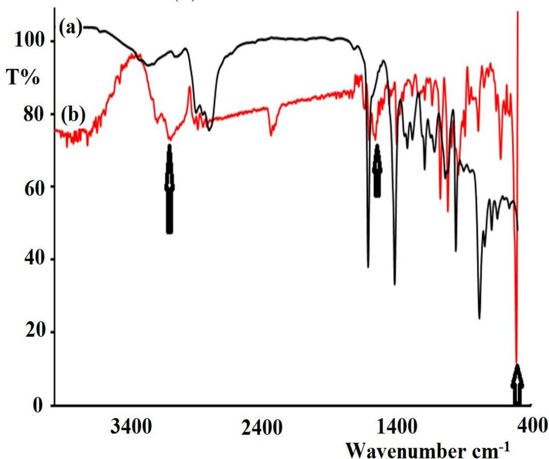
**Fig. (3.6):** IR Spectra of: (a)  $\text{N}_3\text{S}_2$  Ligand and (b) Complex **2**
