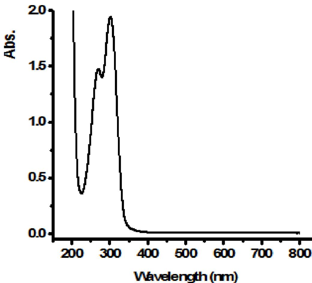
**Fig. (3.19):** UV-Vis Spectra of Free Ligand in Ethanol at Room Temperature
