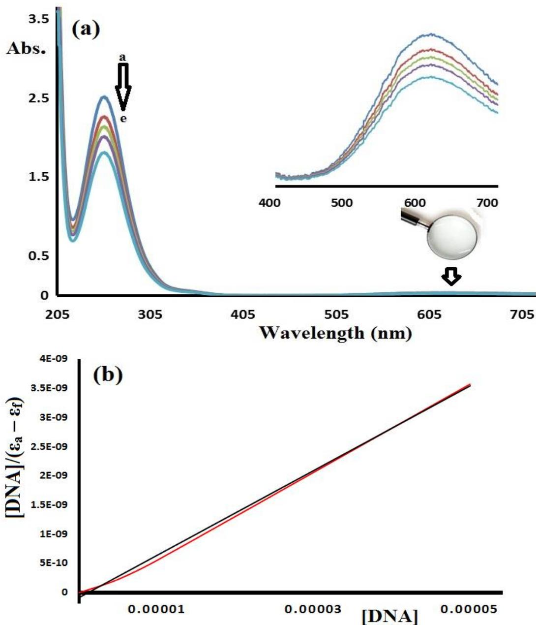
**Fig. (4.1):** (a) UV/Vis. Spectra of  $5.0 \times 10^{-5}$  M of Complex **1** Interacted With 0,  $1.0 \times 10^{-6}$ ,  $5.0 \times 10^{-6}$ ,  $1.0 \times 10^{-5}$  and  $5.0 \times 10^{-5}$  M CT-DNA at RT (a  $\rightarrow$  e). (b) Plot of  $[DNA]/(\epsilon_a - \epsilon_f)$  vs.  $[DNA]$  at 250 nm to determine  $K_b$ .
