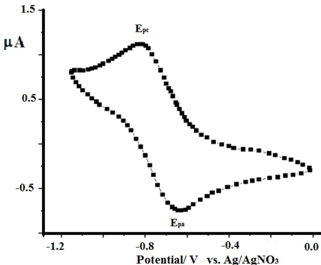
**Fig. (3.12):** CV-Voltammogram of Complex 1 ( $1 \times 10^{-4}$  M) Dissolved in Acetonitrile, 0.1 M TBAHF, Scan Rate 0.10 V/s at RT.
