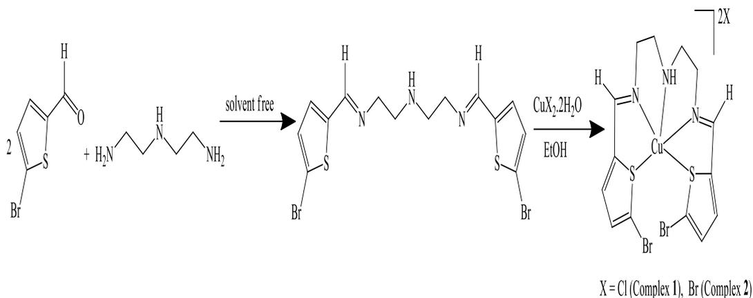
**Scheme 3.** Synthesis of the  $N_3S_2$  Ligand and its Desired Cu(II) Complexes.
