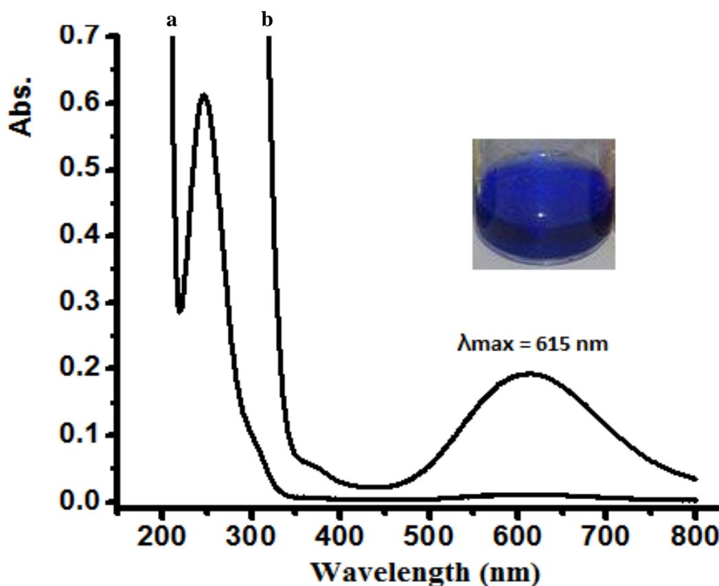
**Fig. (3.9):** UV-Vis Spectra of Complex Dissolved in Water at RT (a)  $5 \times 10^{-5}$  M and (b)  $5 \times 10^{-4}$  M Concentrations.
