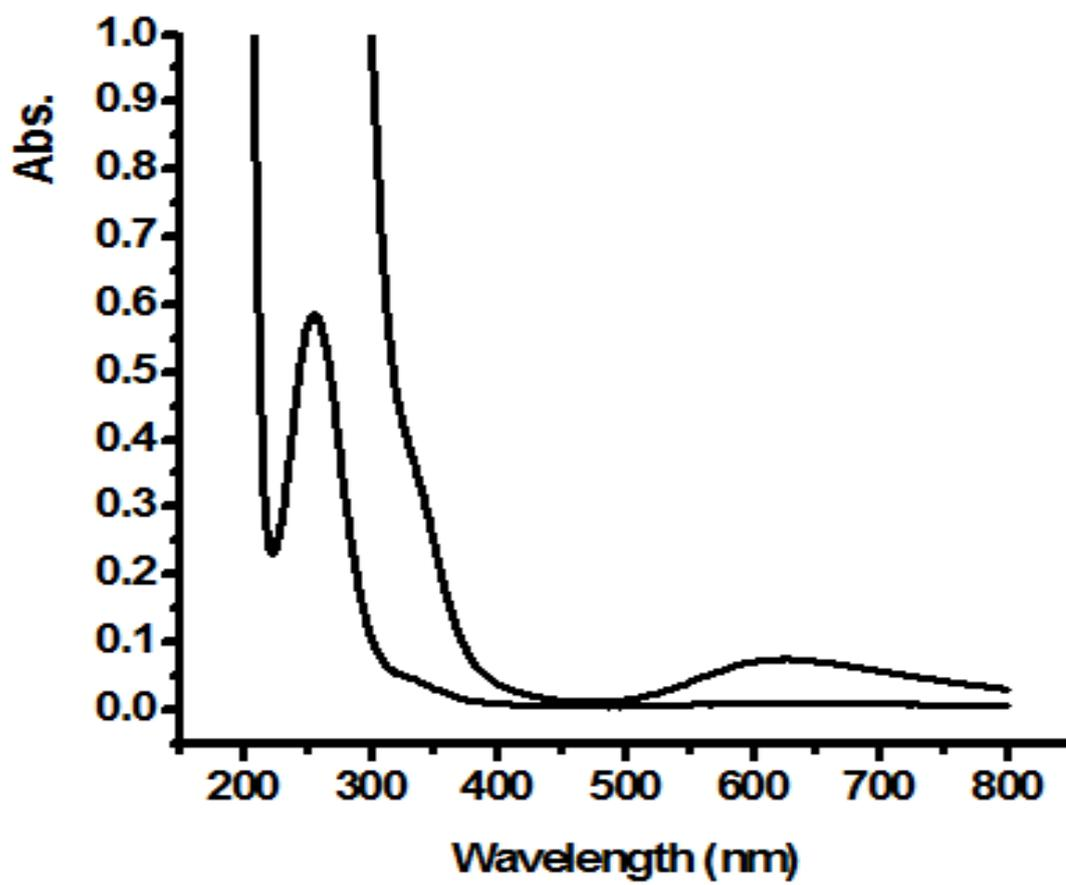
**Fig. (3.20):** UV-Vis Spectra of Complexes 1 Dissolved in Water at Room Temperature
