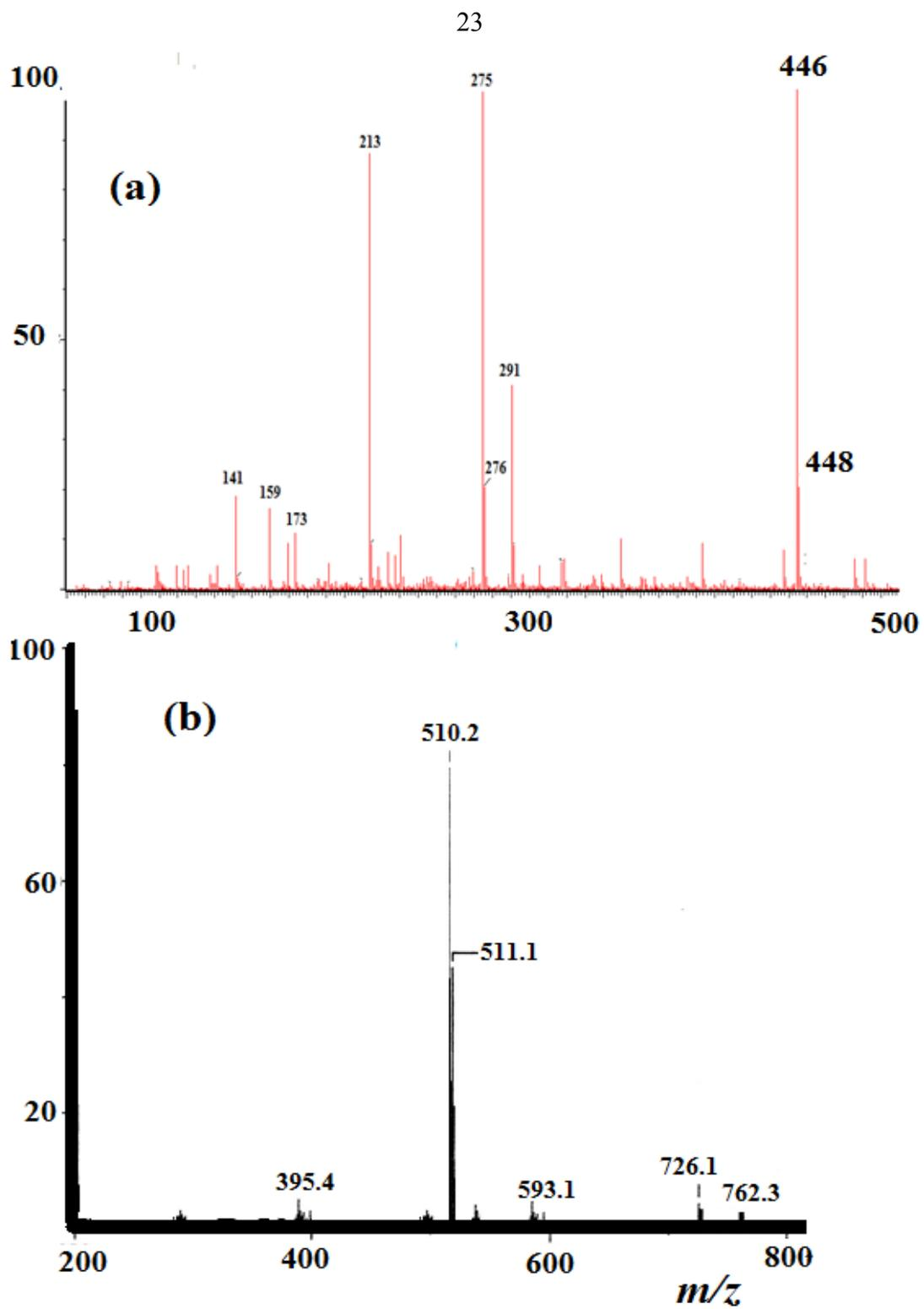
Fig. (3.2): (a) EI-MS Spectrum of the  $N_3S_2$  Ligand and (b) ESI-MS Spectrum of Complex 2.
