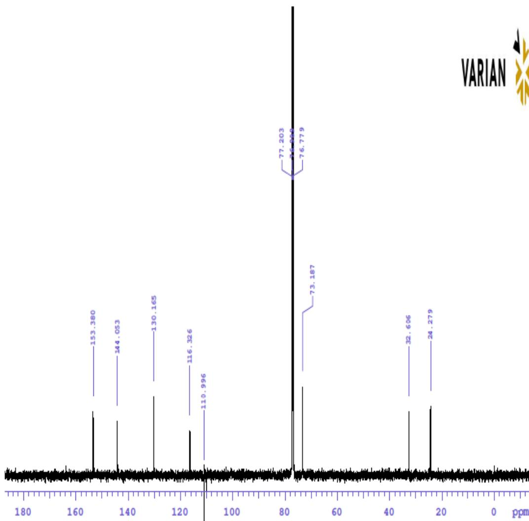
**Fig. (3.17):**  $^{13}\text{C}$  NMR Spectrum of L2 Ligand Dissolved in  $\text{CDCl}_3$  at RT.
