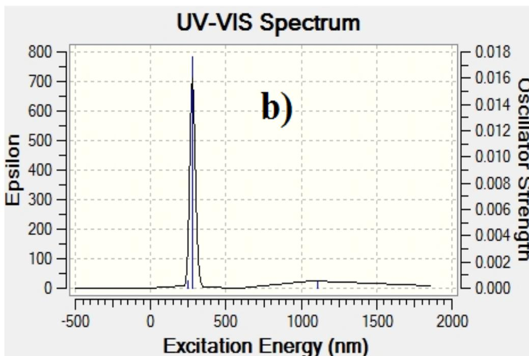
**Fig. (3.8):** UV-Vis. Spectroscopy Spectra of the Ligand a) Experimentally (in Ethanol at RT), and b) TD-DFT/B3LYP/3-311 Theoretically (in Gaseous State).
