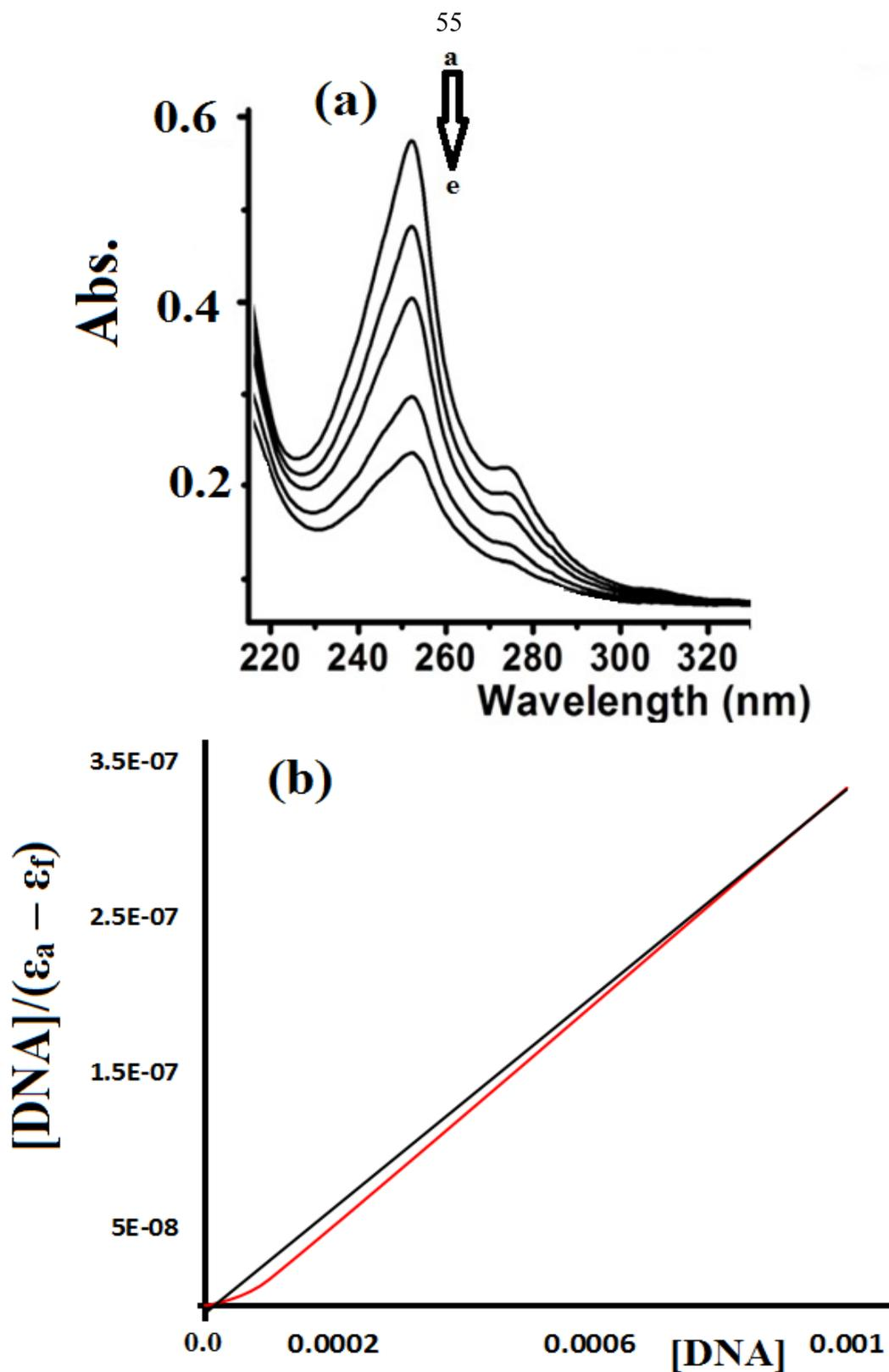
**Fig. (4.2):** (a) UV Spectra of  $1.0 \times 10^{-5}$  M of Complex **2** Interacted With 0,  $1.0 \times 10^{-6}$ ,  $1.0 \times 10^{-5}$ ,  $1.0 \times 10^{-4}$  and  $1.0 \times 10^{-3}$  M CT-DNA at RT (a→e). (b) Plot of  $[DNA]/(\epsilon_a - \epsilon_f)$  vs.  $[DNA]$  at 255 nm to Determine the Intrinsic Binding Constant
