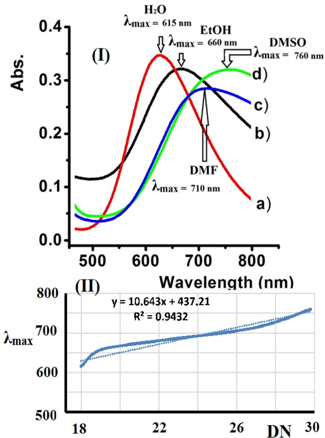
**Fig. (3.10):** (I) Absorption Spectra of Complex 2 Dissolved in Selected Solvents, (II) Dependence of  $\lambda_{\max}$  of Complex 2 on the Solvent Gutmann's Donor Number Values (DN).
