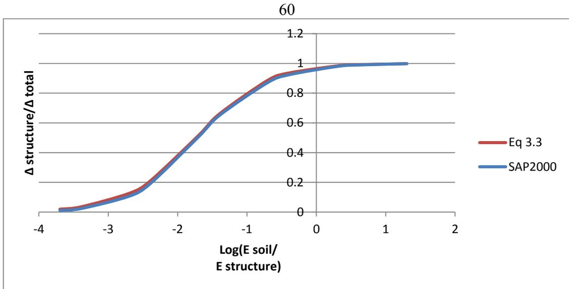
**Figure 3.16:** Comparison between the finite element results and the equation 3.3 results for  $\frac{\Delta_{\text{structure}}}{\Delta_{\text{total}}}$  curve.
