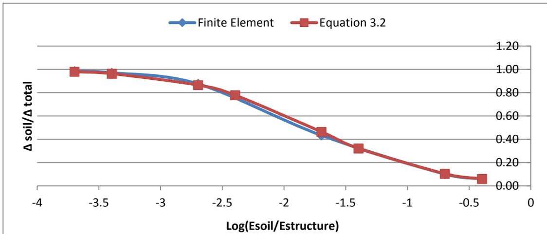
**Figure 4.5:** Comparison between the finite elements method and Equation 3.2 results for frame with  $\frac{c}{l}$  ratio equals 0.2 and  $\frac{l}{d}$  value equals 3 and G value of 0.833.
