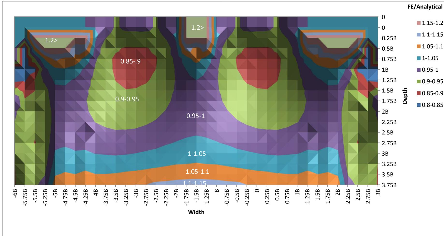
**Figure 2.10:** Comparison between the analytical and the finite element methods as a ratio to the analytical results for two area loads.
