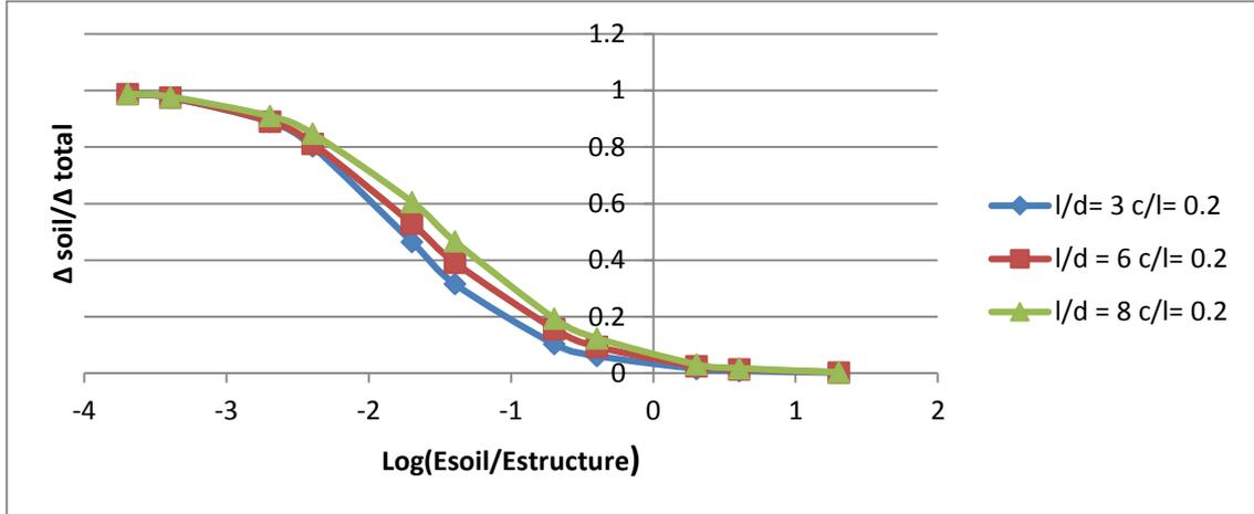
**Figure 3.12:** The change of  $\frac{\Delta_{soil}}{\Delta_{total}}$  curves for  $\left(\frac{c}{l}\right)$  value 0.2 and various  $\left(\frac{l}{d}\right)$  values.
