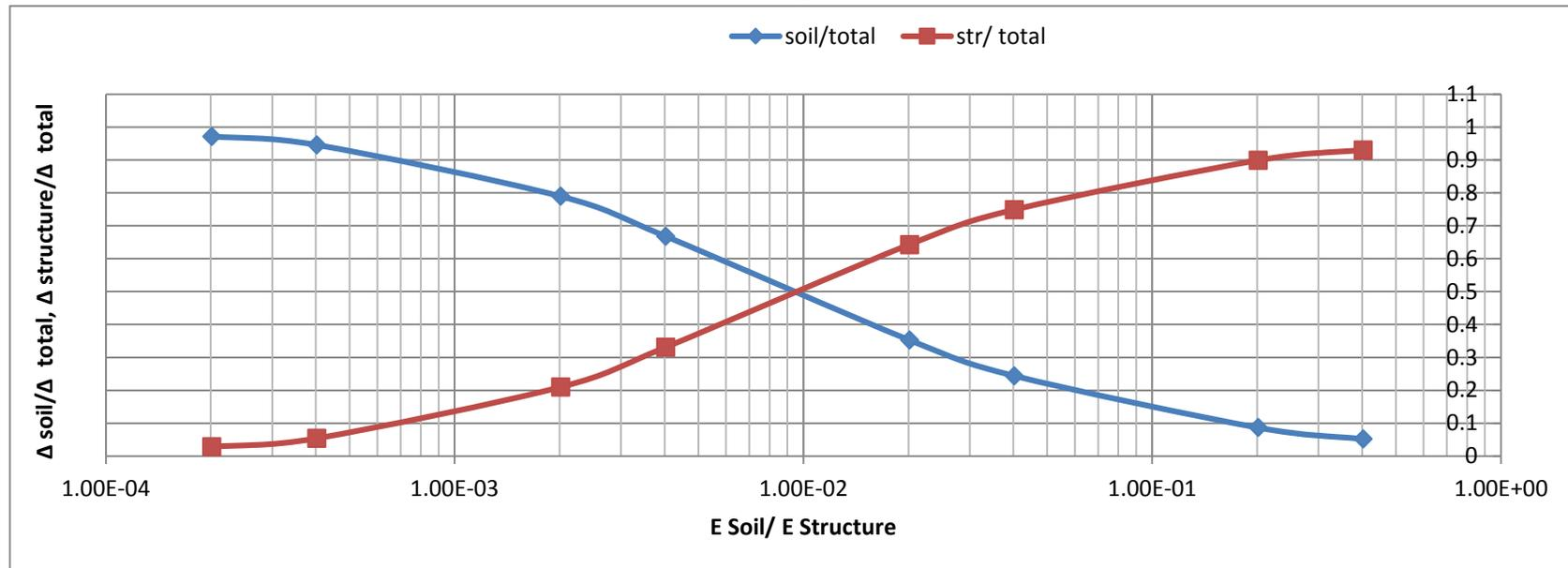
**Figure 3.4 :** A representative diagram shows  $\Delta_{\text{soil}}/\Delta_{\text{total}}$  and  $\Delta_{\text{structure}}/\Delta_{\text{total}}$  curves for the model with values  $(l/d) = 6$  and  $(c/l) = 0.15$ .
