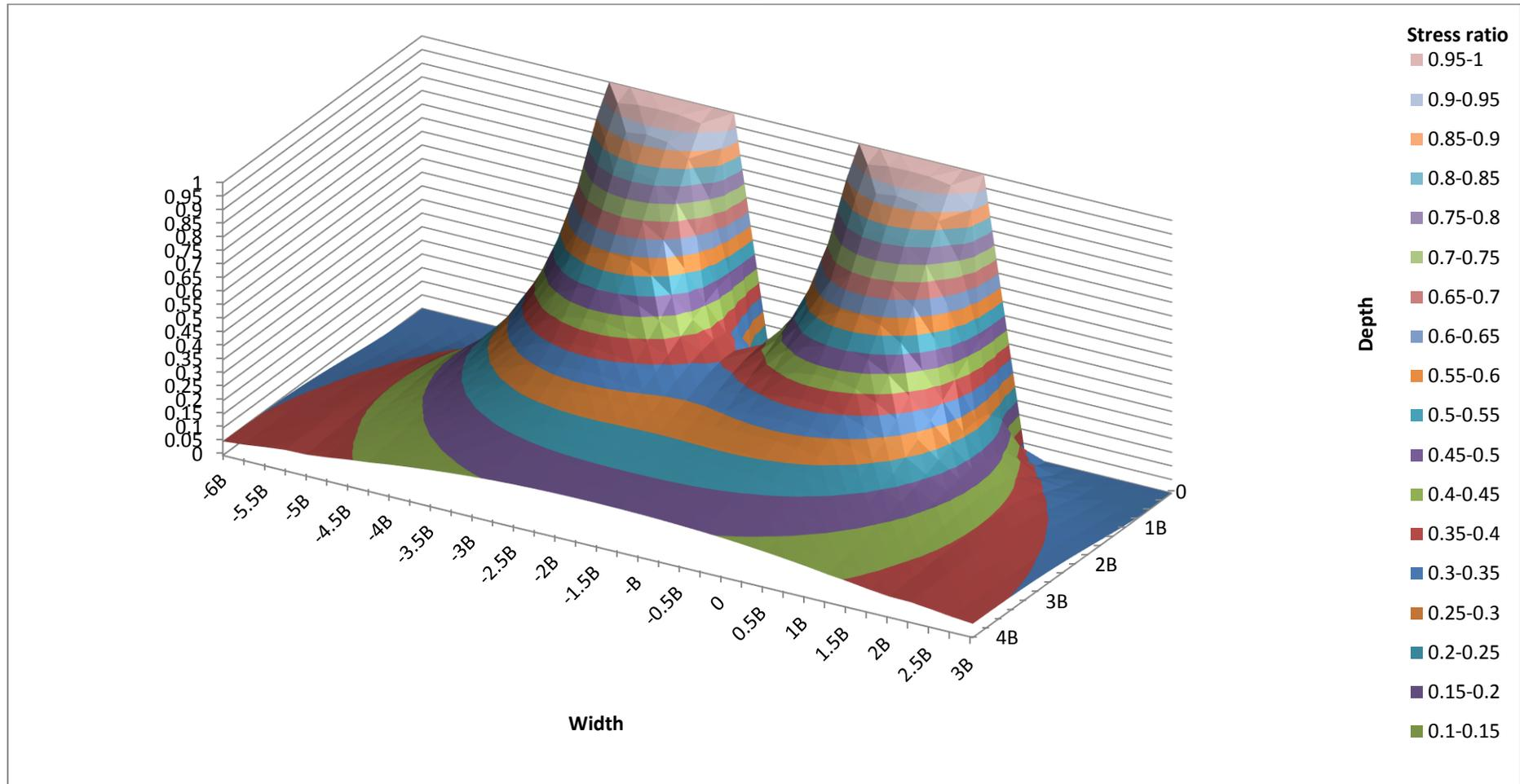
**Figure 2.8:** Stress diagram for two area loads due to analytical calculations.
