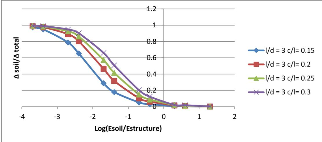
Figure 3.6: The change of  $\frac{\Delta_{soil}}{\Delta_{total}}$  curves for  $\left(\frac{l}{d}\right)$  value 3 and various  $\left(\frac{c}{l}\right)$  values.
