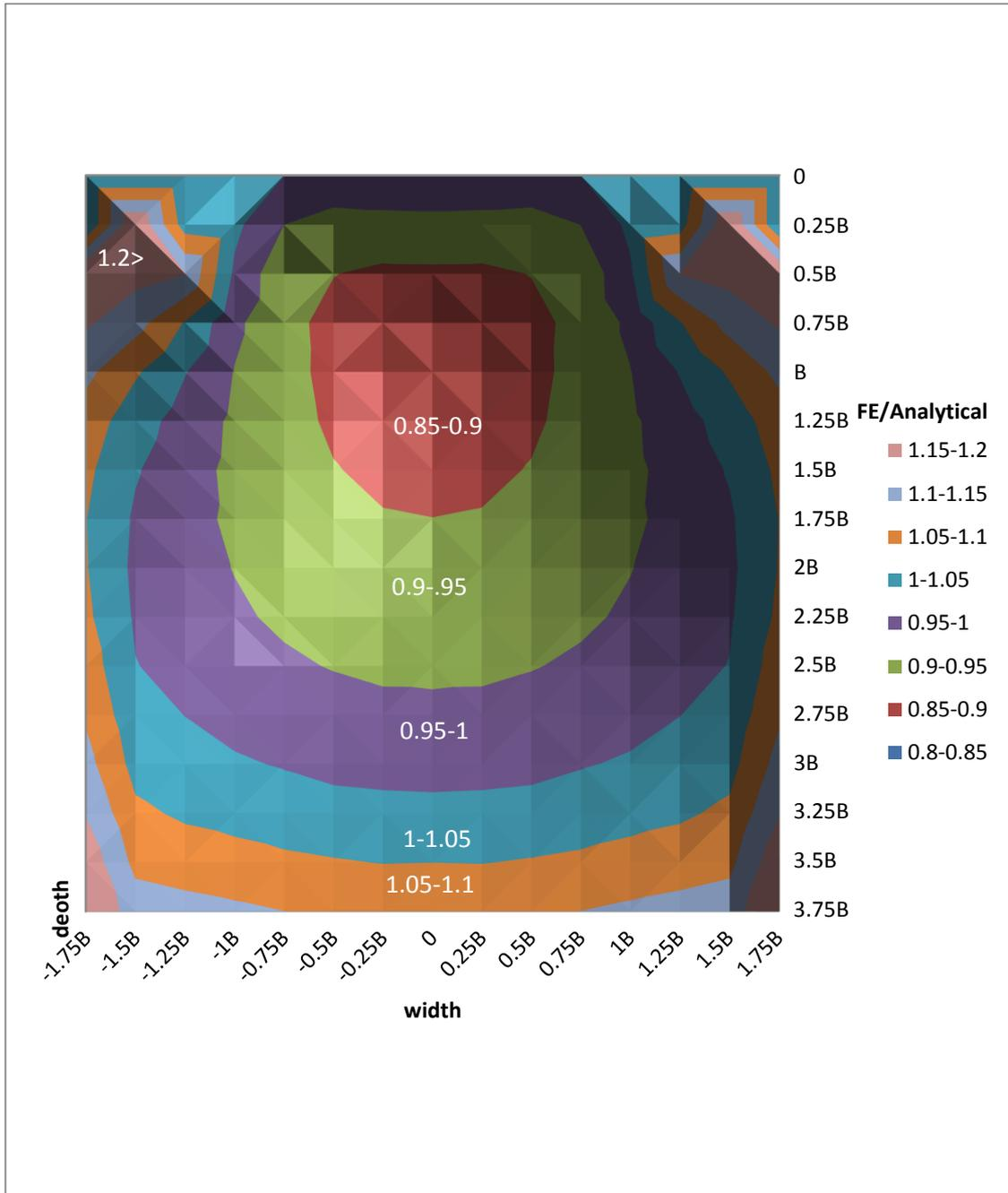
**Figure 2.5:** Comparison between the analytical and the finite element methods as a ratio to the analytical results for an area load.
