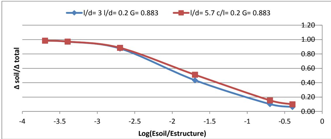
**Figure 4.8:** The change in the curves with the change of  $\frac{l}{d}$  ratio, considering the other variables are constants.
