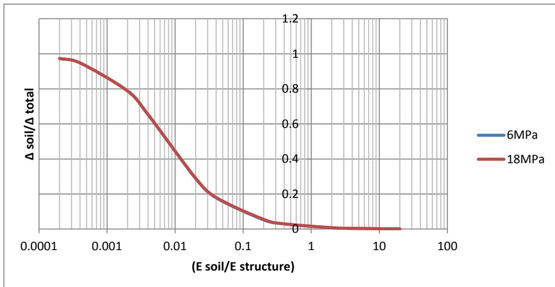
**Figure 3.13:** The change of  $\frac{\Delta_{\text{soil}}}{\Delta_{\text{total}}}$  curves for varies values of stress, where  $\sigma$  is stress unit.
