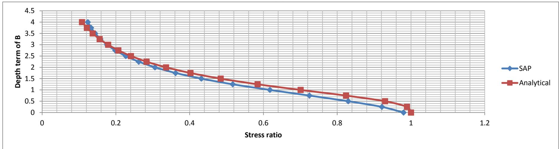
Figure 2.7: Comparison between the analytical stress and the finite element stress under the center of the area load.
