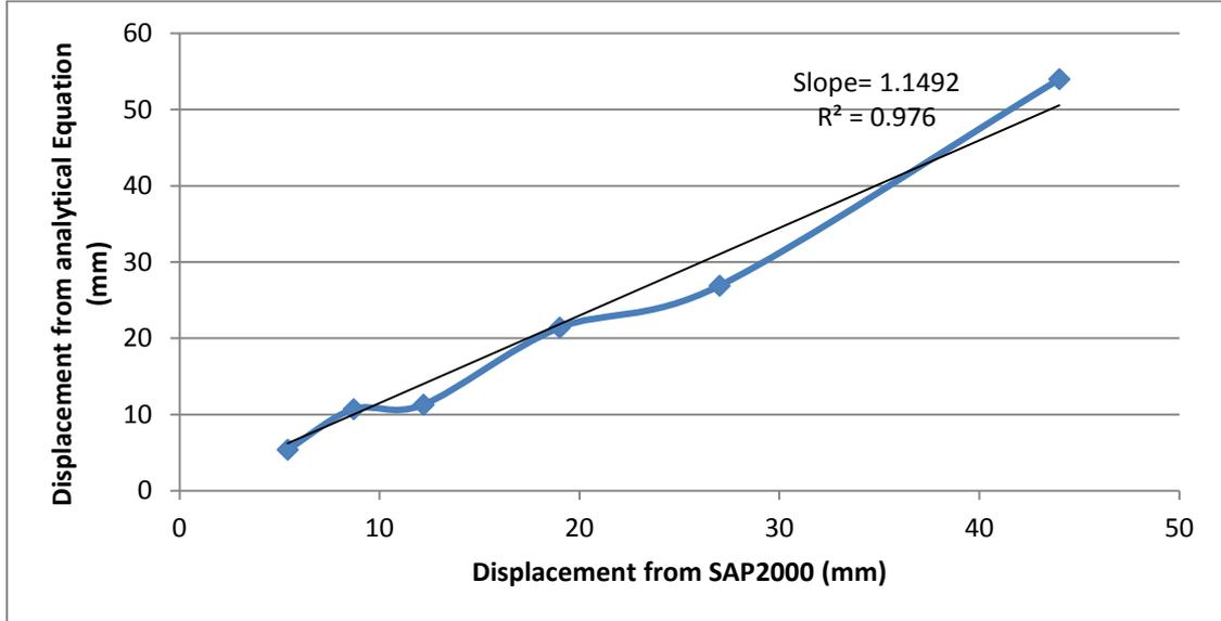
**Figure 2.2:** Displacement of soil from SAP2000 versus the displacement from the analytical equation 2.2 and 2.3.
