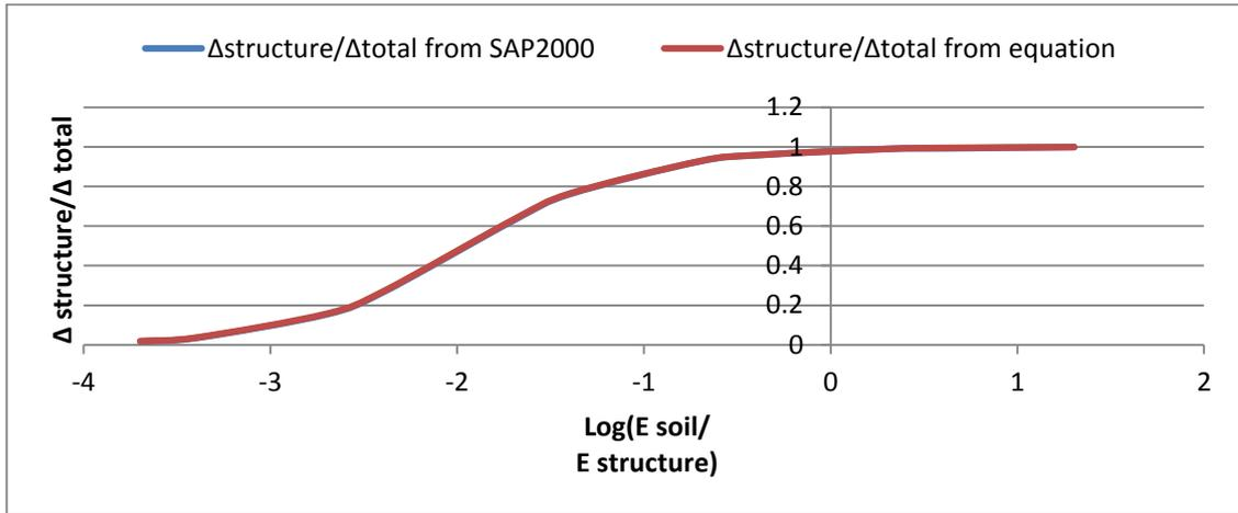
**Figure 3.21:** Comparison curves between the finite element results and equation 3.9 results for the  $\frac{\Delta_{\text{structure}}}{\Delta_{\text{total}}}$  values for a model with height of 1.5  $l$  of the previous experiments.
