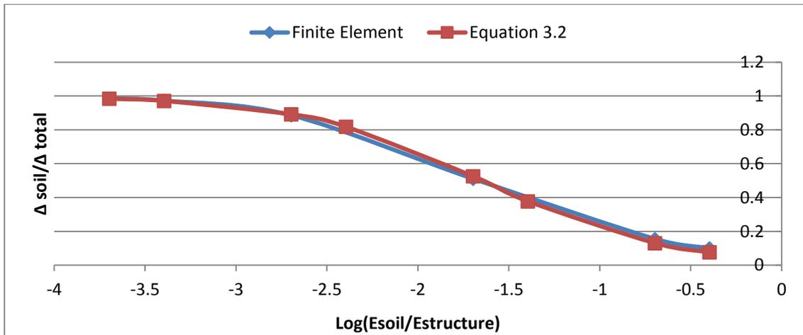
**Figure 4.9:** Comparison between the finite elements method and Equation 3.2 results for frame with  $\frac{c}{l}$  ratio equals 0.2 and  $\frac{l}{d}$  value equals 5.7 and G value of 0.833.
