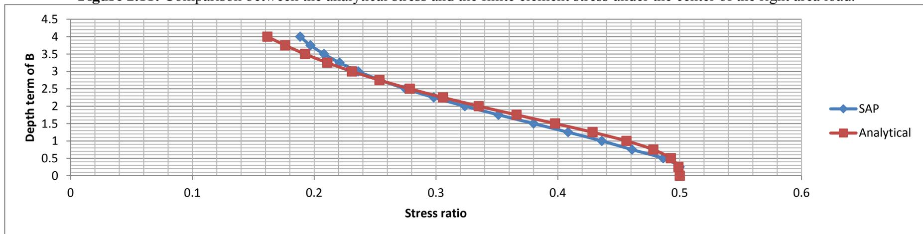
**Figure 2.12:** Comparison between the analytical stress and the finite element stress under the left corner of the right area load.
