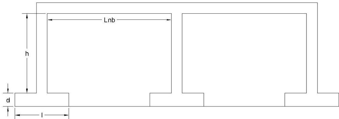
**Figure 4.2:** The frame used as model with the parameters used in the simulation.
