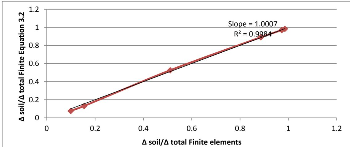
**Figure 4.10:** Comparison of  $\frac{\Delta_{\text{soil}}}{\Delta_{\text{total}}}$  results of finite elements versus Equation 3.2.
