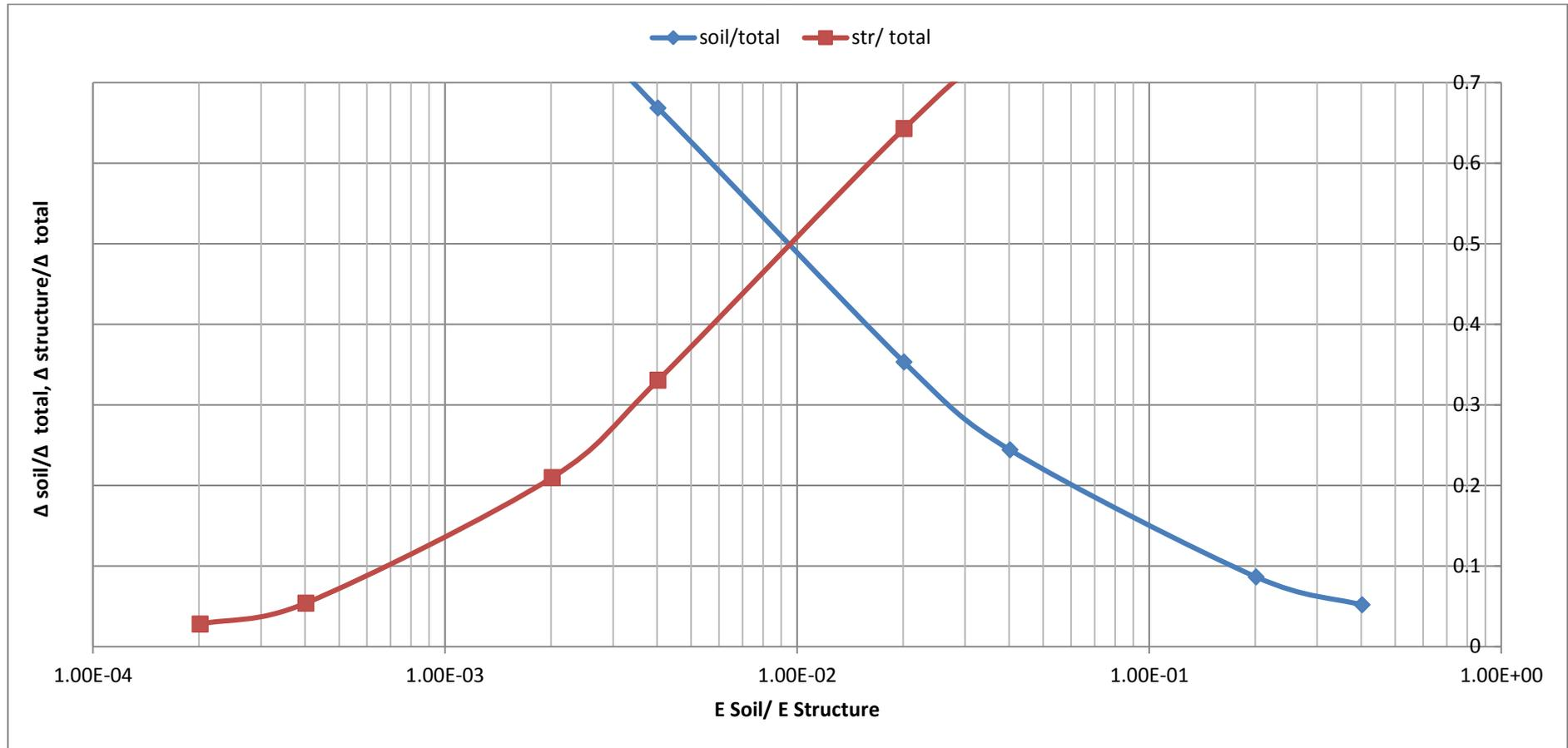
**Figure 3.5:** representative zoomed diagram shows  $\Delta_{\text{soil}}/\Delta_{\text{total}}$  and  $\Delta_{\text{structure}}/\Delta_{\text{total}}$  curves for the model with values  $(l/d) = 6$  and  $(c/l) = 0.15$ .
