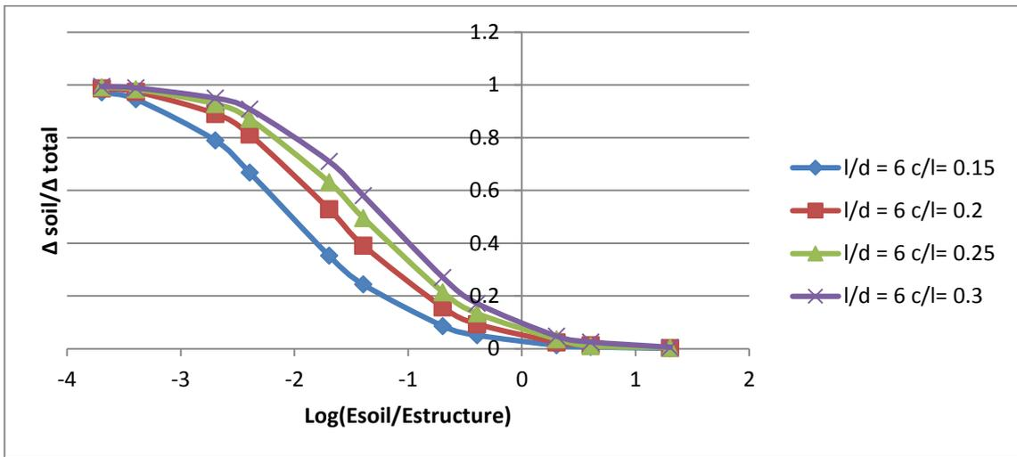
Figure 3.7: The change of  $\frac{\Delta_{soil}}{\Delta_{total}}$  curves for  $\left(\frac{l}{d}\right)$  value 6 and various  $\left(\frac{c}{l}\right)$  values.
