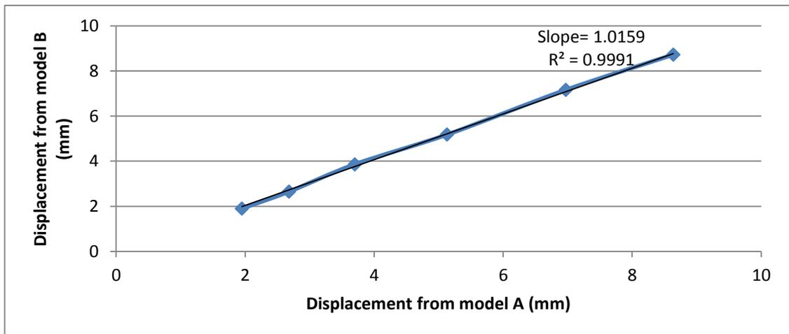
**Figure 2.1:** The displacement from model A versus the displacement from model B, as an indication of the mesh size effect on the displacement of the multi-nodded elements.
