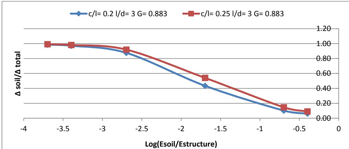
**Figure 4.4:** The change in the curves with the change of  $\frac{c}{l}$  ratio, considering the other variables are constants.
