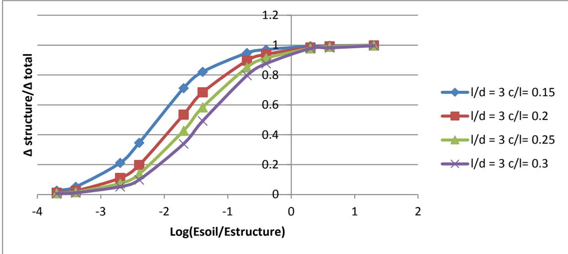
Figure 3.9: the change of  $\frac{\Delta_{structure}}{\Delta_{total}}$  curves for value  $\left(\frac{l}{d}\right) = 3$  and various  $\left(\frac{c}{l}\right)$  values
