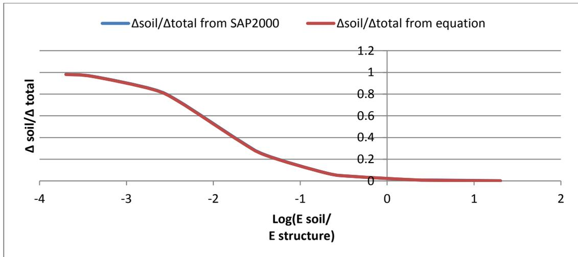
**Figure 3.20:** Comparison curves between the finite element results and equation 3.8 results for the  $\frac{\Delta_{soil}}{\Delta_{total}}$  values for a model with height of 1.5  $l$  of the previous experiments.
