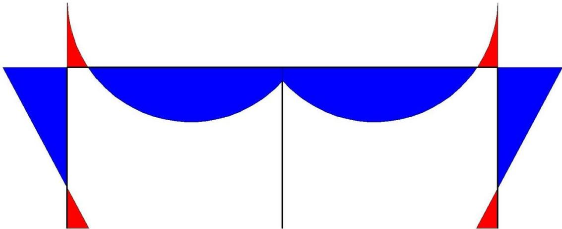
**Figure 1.5:** General sketch of bending moment diagram for two spans frame with large settlement in the middle column.
