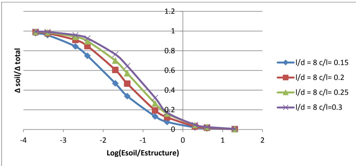
Figure 3.8: The change of  $\frac{\Delta_{soil}}{\Delta_{total}}$  curves for  $\left(\frac{l}{d}\right)$  value 8 and various  $\left(\frac{c}{l}\right)$  values.
