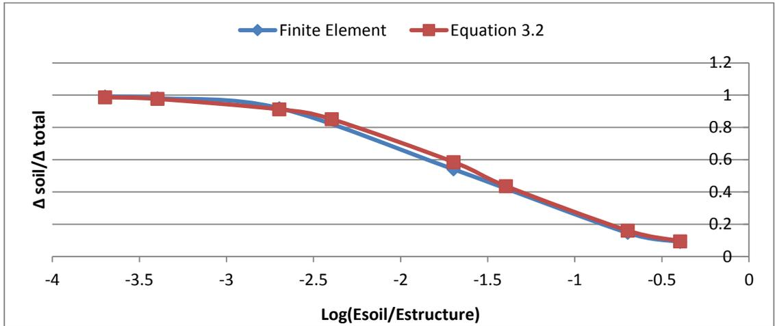
**Figure 4.6:** Comparison between the finite elements method and Equation 3.2 results for frame with  $\frac{c}{l}$  ratio equals 0.25 and  $\frac{l}{d}$  value equals 3 and G value of 0.833.
