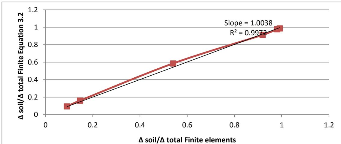
**Figure 4.7:** Comparison of  $\frac{\Delta_{soil}}{\Delta_{total}}$  results of finite elements versus Equation 3.2.
