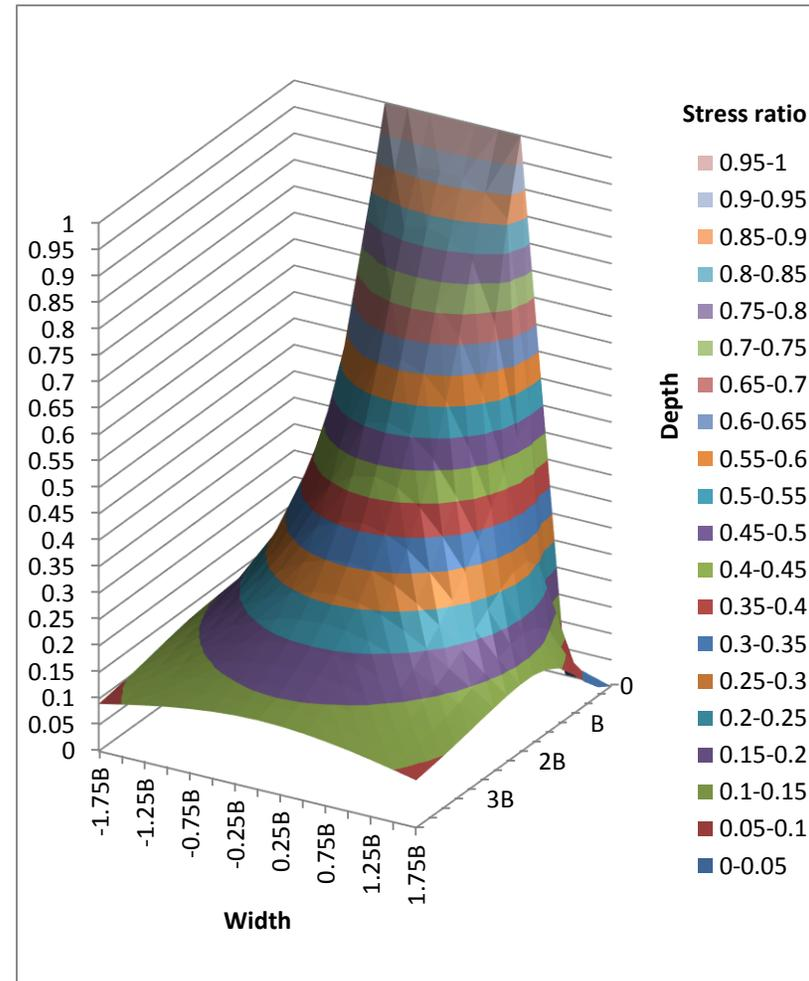
**Figure 2.3:** Stress curves for an area load due to finite element analysis using SAP2000.
