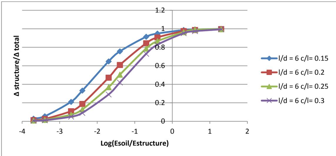
Figure 3.10: the change of  $\frac{\Delta_{structure}}{\Delta_{total}}$  curves for value  $\left(\frac{l}{d}\right) = 6$  and various  $\left(\frac{c}{l}\right)$  values
