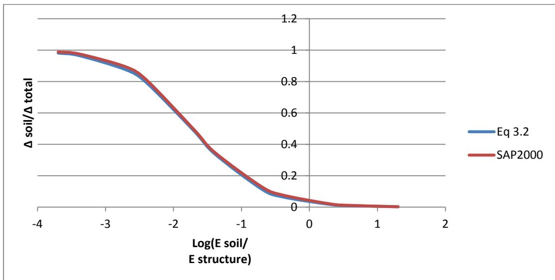
**Figure 3.17:** Comparison between the finite element results and the equation 3.2 results for  $\frac{\Delta_{\text{soil}}}{\Delta_{\text{total}}}$  curve.
