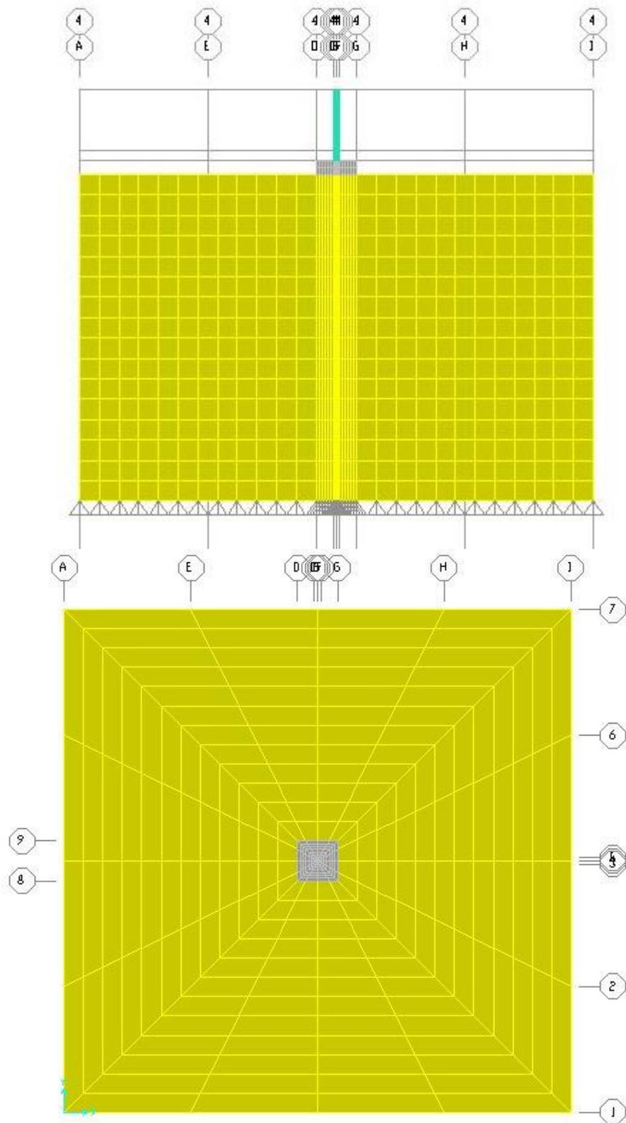
**Figure 3.2:** Representative meshed model using the finite elements tool SAP2000.
