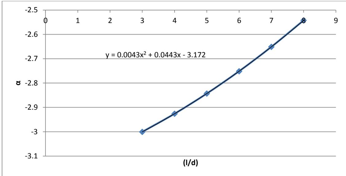
**Figure 3.15:** A curve representing the relationship between  $\left(\frac{l}{d}\right)$  and the variable  $\alpha$ .
