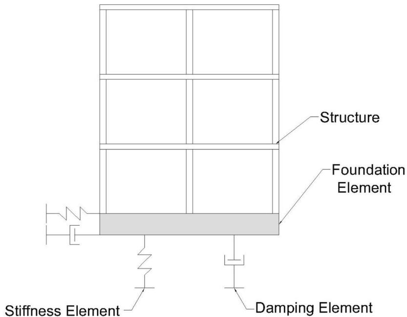
**Figure 1.2:** Typical substructure approach model.
