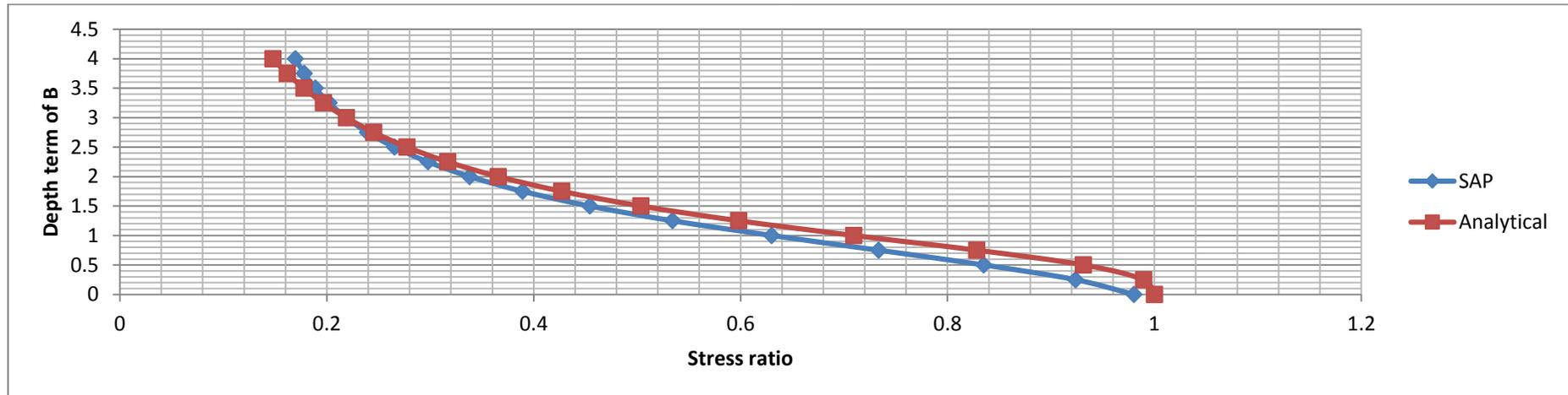
**Figure 2.11:** Comparison between the analytical stress and the finite element stress under the center of the right area load.
