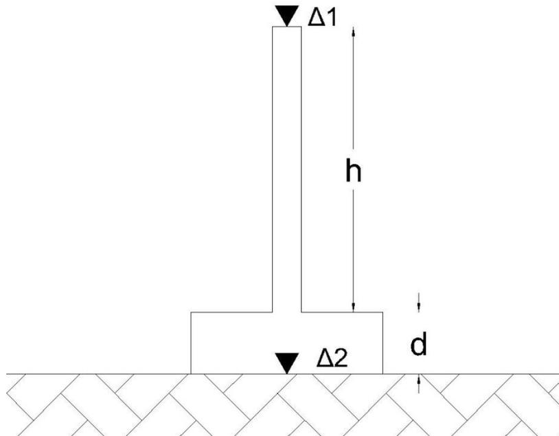
**Figure 3.3:** Total displacement ( $\Delta_1$ ), and soil displacements ( $\Delta_2$ ).
