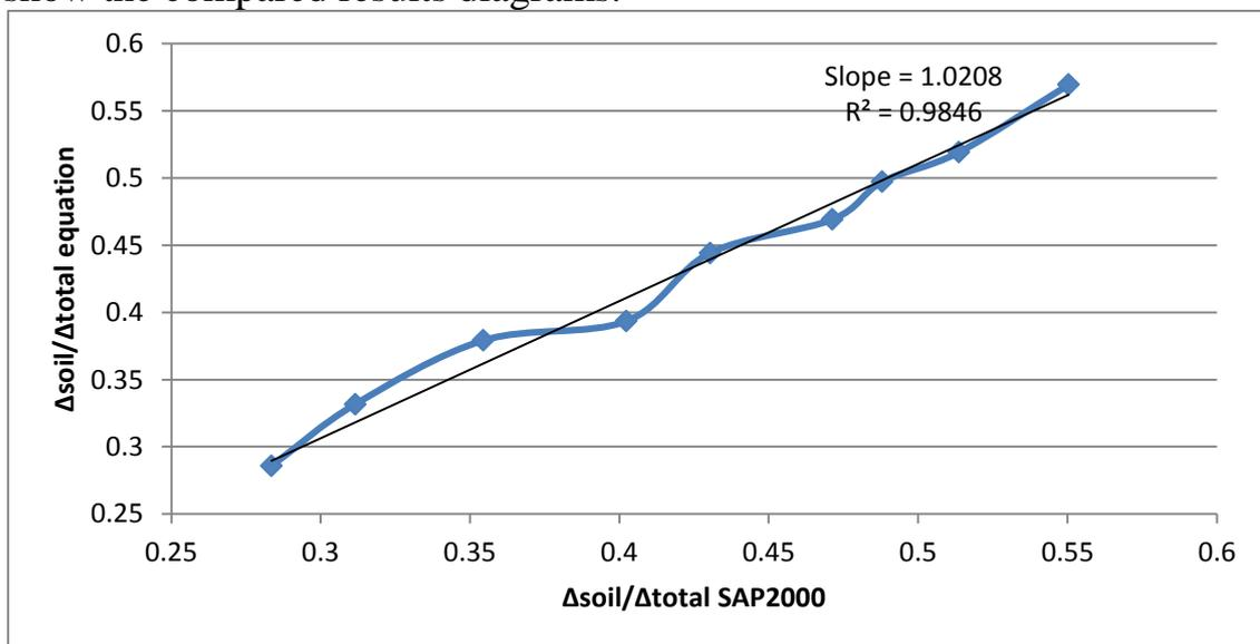
**Figure 3.18:**  $\frac{\Delta_{soil}}{\Delta_{total}}$  from SAP2000 versus  $\frac{\Delta_{soil}}{\Delta_{total}}$  from Equation 3.2.
