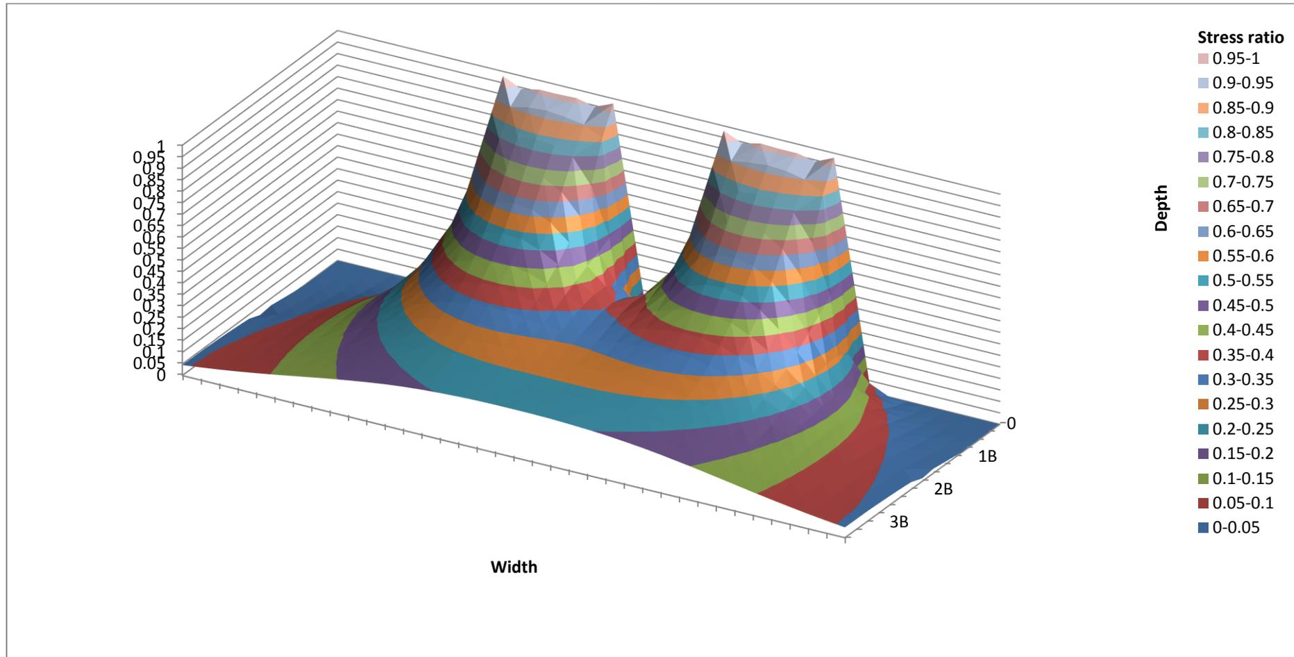
**Figure 2.9:** Stress diagram for two area loads due to finite element calculations
