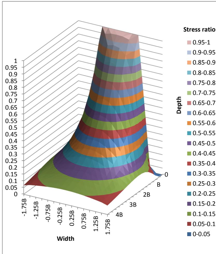
**Figure 2.4:** Stress curves for an area load due to analytical calculations.
