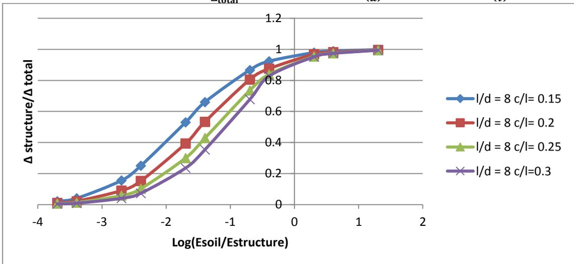
Figure 3.11: the change of  $\frac{\Delta_{structure}}{\Delta_{total}}$  curves for value  $\left(\frac{l}{d}\right) = 8$  and various  $\left(\frac{c}{l}\right)$  values
