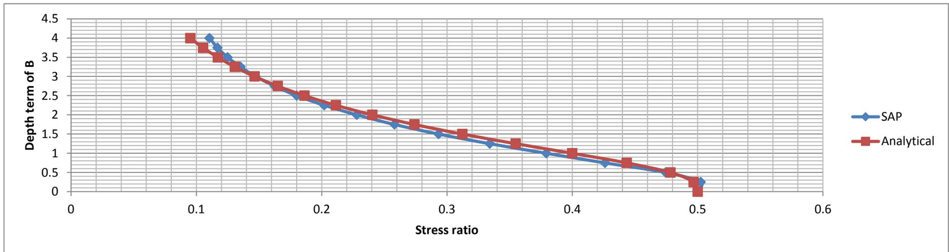
Figure 2.6: Comparison between the analytical stress and the finite element stress under the corner of the area load.
