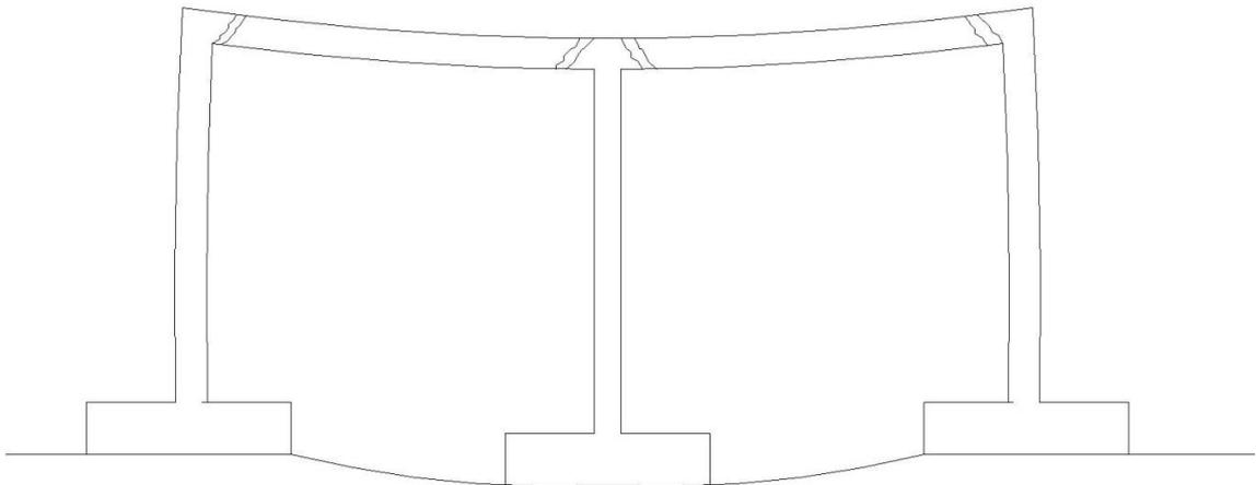
**Figure 1.3:** Two-span frame with non-uniform settlement in the middle footing.
