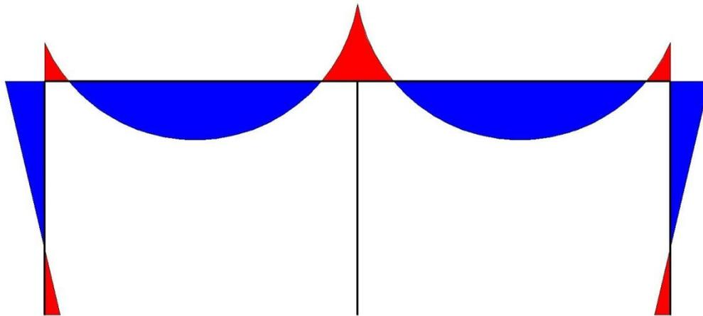
**Figure 1.4:** General sketch of bending moment diagram for two spans frame with fixed soil.
