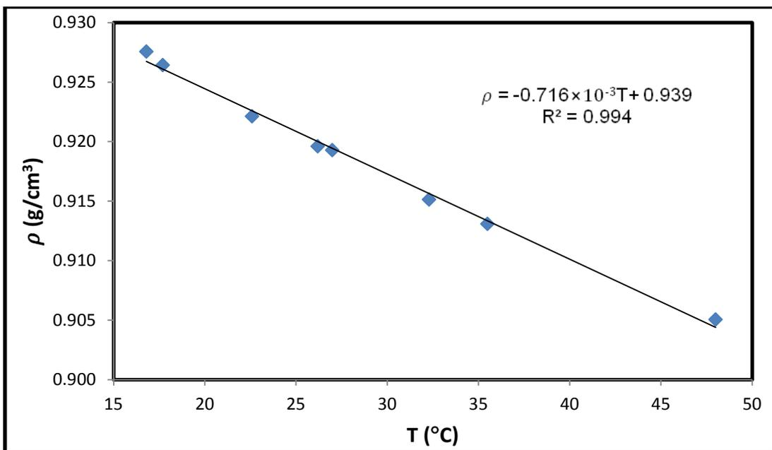
Fig. (A.6): The measured density for Jenin sample from 2010 crop versus temperatures
