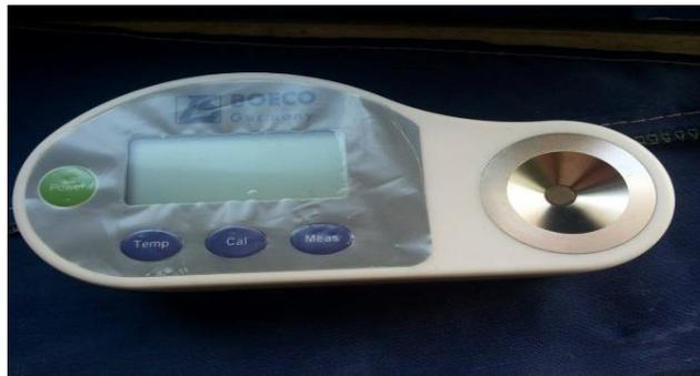
**Fig. (3.3):** A digital refractometer the way 2sABBE
