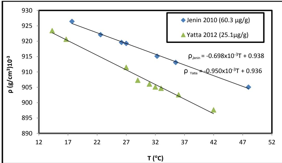
**Fig.(4.11):** The effect of two different concentrations of iron (Fe) on the density as function of temperature
