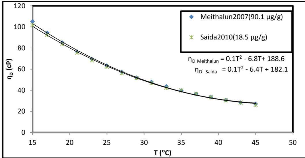
**Fig. (4.14):** The effect of the highest and lowest concentration of iron Fe on viscosity as function of temperature
