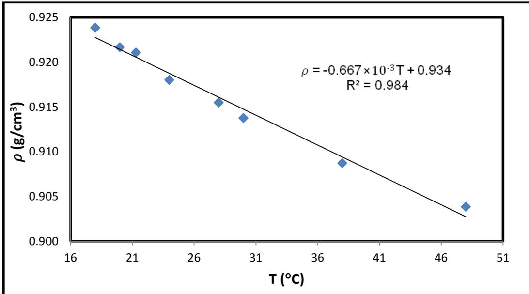
**Fig. (A.3):** The measured density for Meithalun sample from 2010 crop versus temperatures
