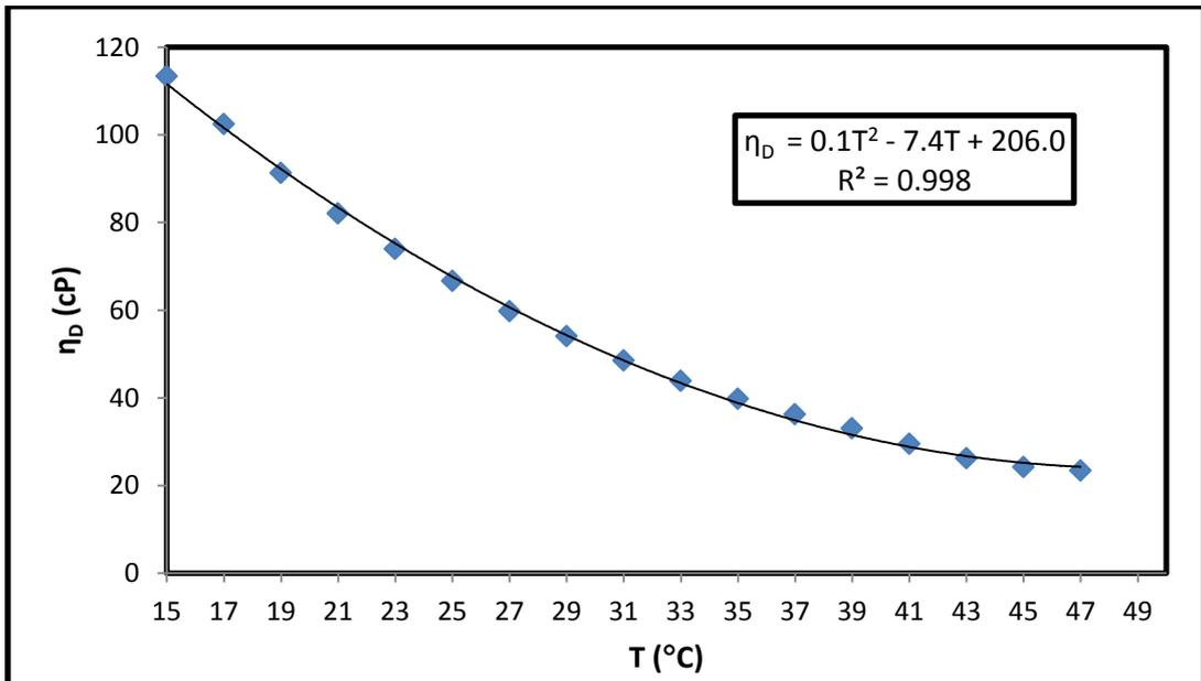
**Fig.(B.10):** Dynamic viscosity versus temperatures of Jenin sample 2007crop
