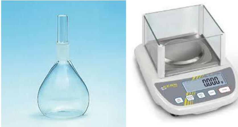
**Fig. (3.2):**Pycnometer and HR-200 analytical balance
