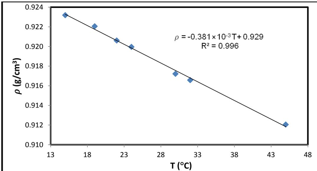
**Fig. (A.4):** The measured density for Saida sample from 1997 crop versus temperatures
