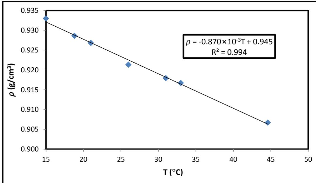
**Fig.(4.1):** The measured density for Saida sample from 2012 crop versus temperatures. The density as function of temperatures gives a linear relation, the negative slope of the equation in Fig.(4.1) indicates rate change of density with temperature is of the form  $\rho = -0.870 \times 10^{-3}T + 0.925$ .
