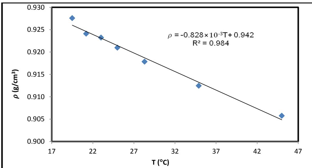
**Fig. (A.2):** The measured density for Yasid sample from 2011 crop versus temperatures
