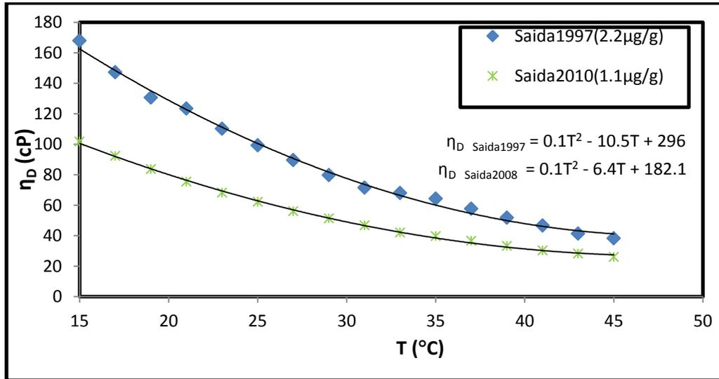
**Fig. (4.13):** The effect of the highest and lowest concentrations of copper Cu on viscosity as function of temperature
