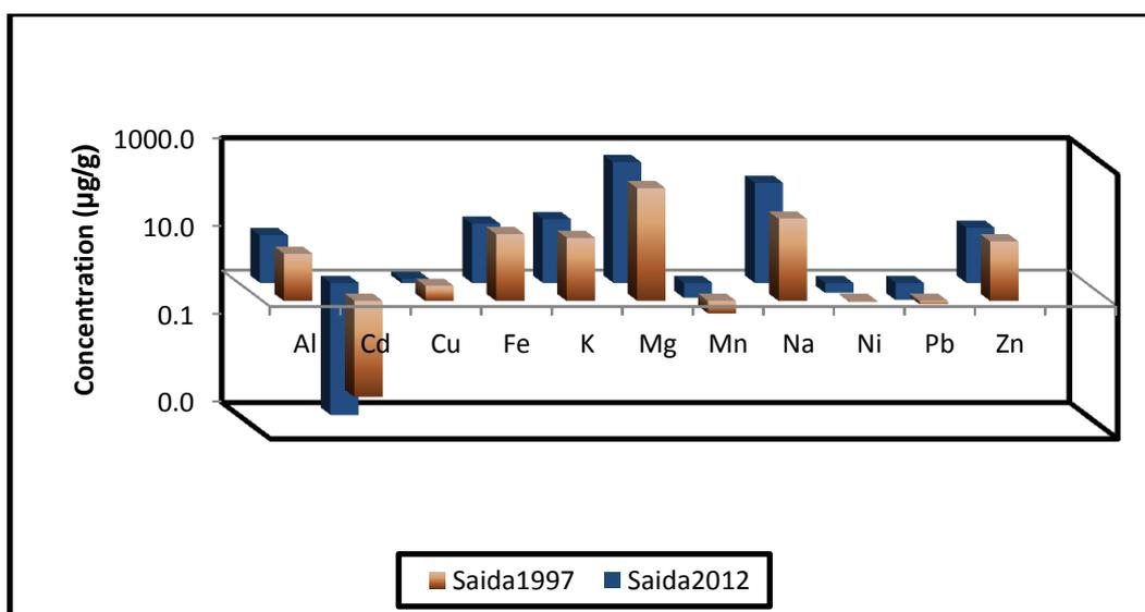
**Fig.(C.2):** The comparison between the levels of metals for two different storage age olive oil samples of same region(Saida)
