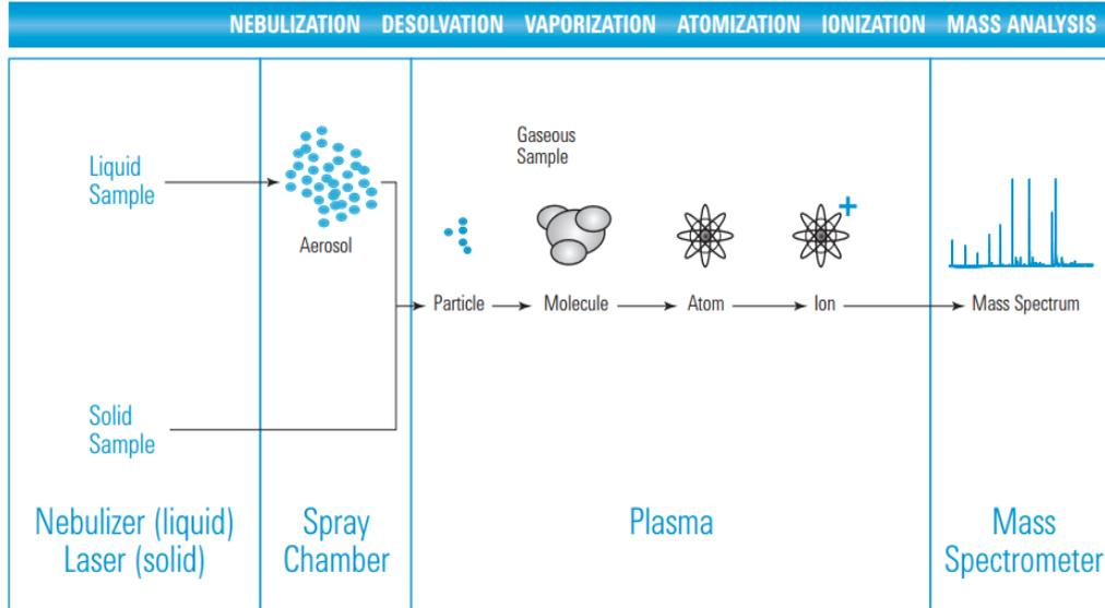
**Fig. (2.1):** The inductively coupled plasma mass spectrometry ICP-MS processes (Agilent, 2005).
