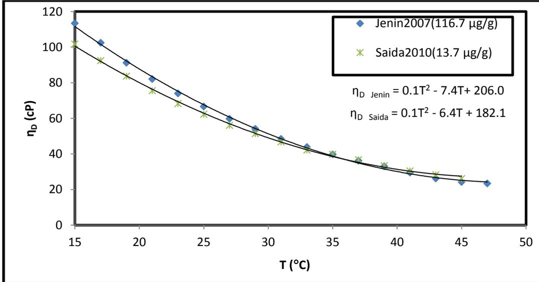
**Fig. (4.15):** The effect of the highest and lowest concentrations of zinc Zn on viscosity as function of temperature
