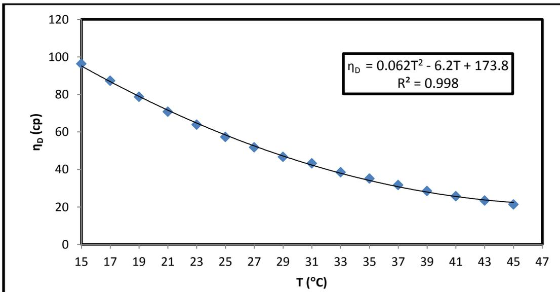
**Fig.(B.2):** Dynamic viscosity versus temperatures of Yasid sample 2011 crop
