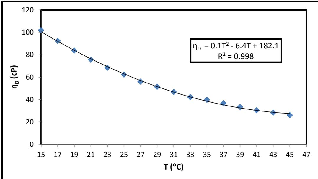
**Fig.(B.7):** Dynamic viscosity versus temperatures of Saida sample 2010 crop
