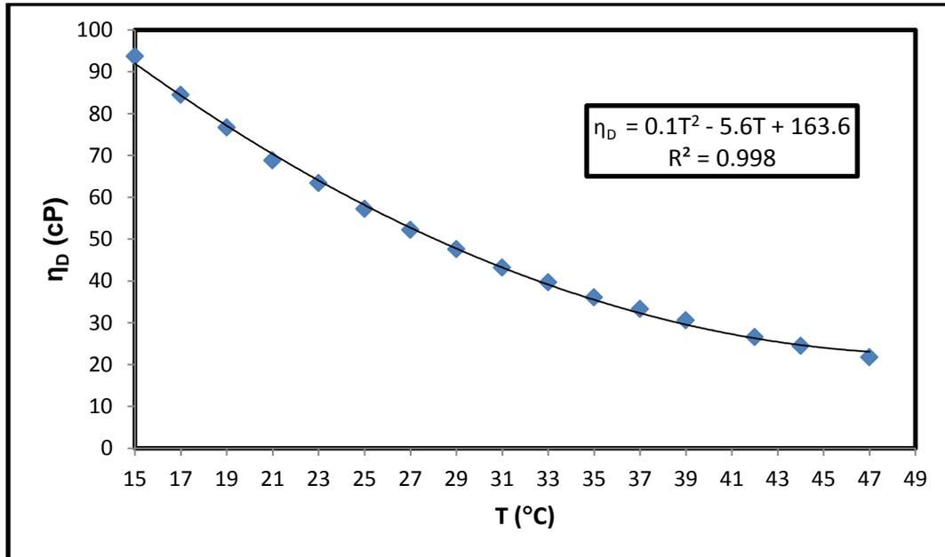
**Fig.(B.11):** Dynamic viscosity versus temperatures of Jenin sample 2010 crop
