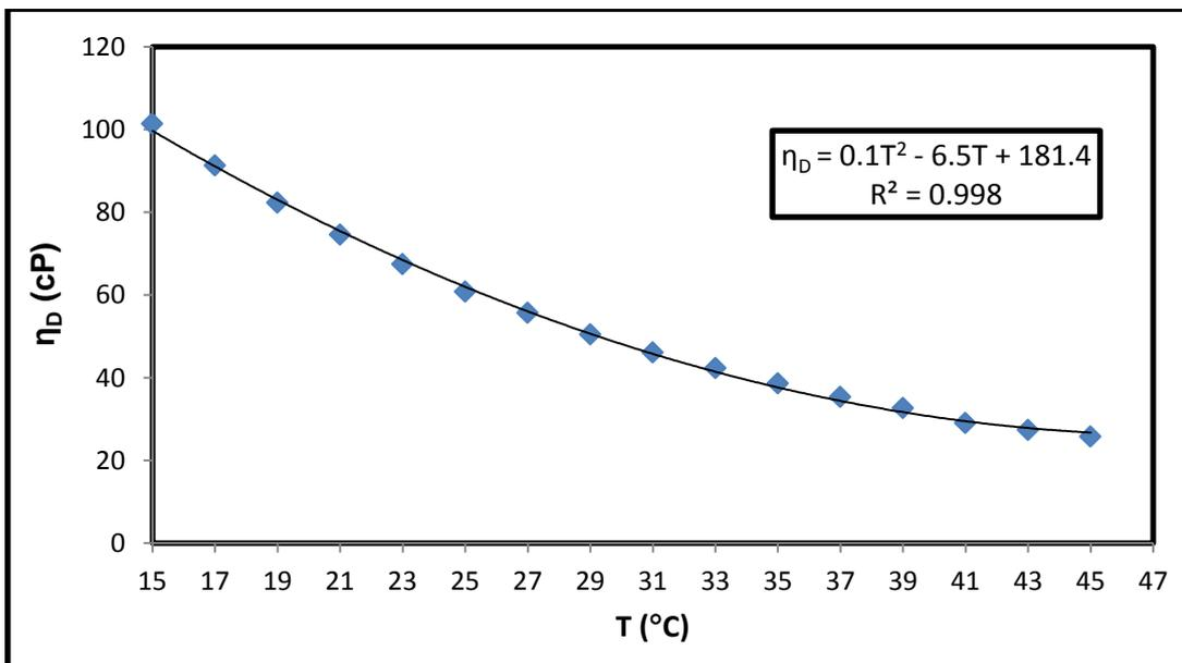
**Fig.(B.6):** Dynamic viscosity versus temperatures of Saida sample 2008 crop
