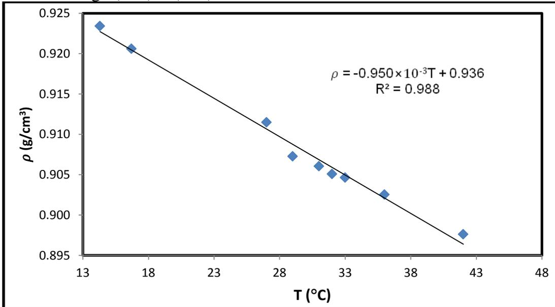
**Fig.(A.1):** The measured density for Yatta sample from 2012 crop versus temperatures
