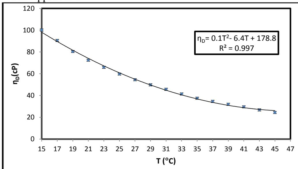
**Fig.(4.3): Dynamic viscosity versus temperatures of Saida sample of 2012 crop**
