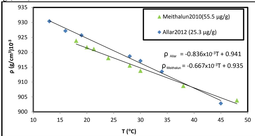
**Fig.(4.12):** The effect of two different concentrations of zinc Zn on the density as function of temperature
