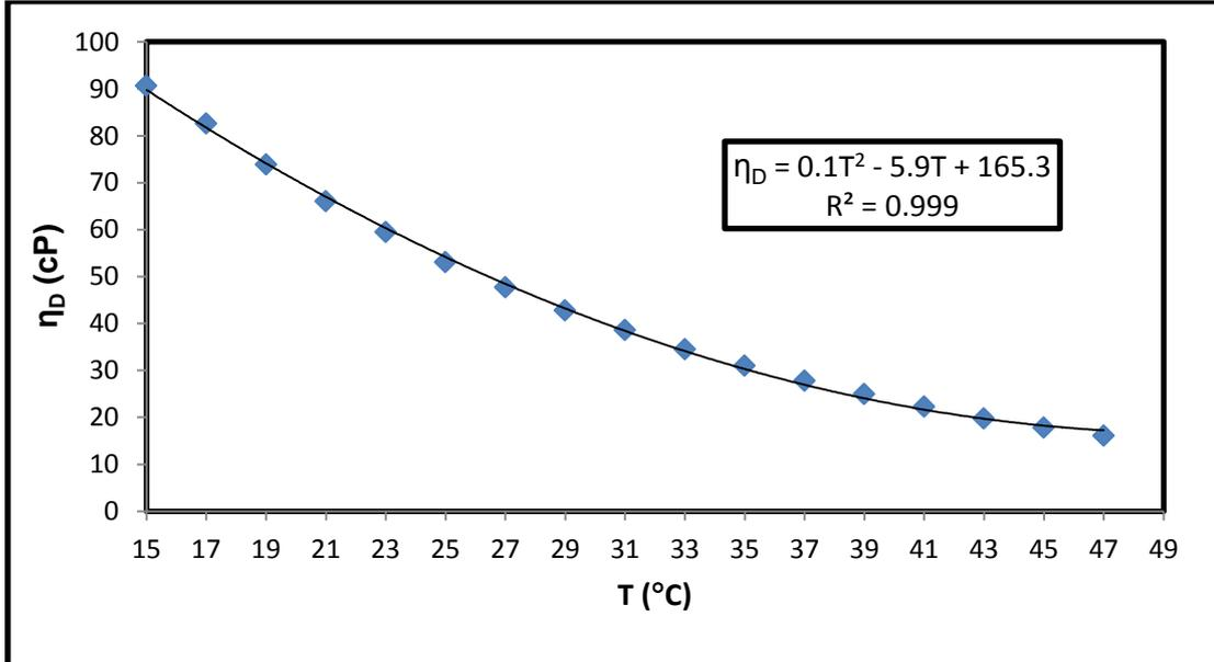
**Fig.(B.9):** Dynamic viscosity versus temperatures of Allar sample 2012crop
