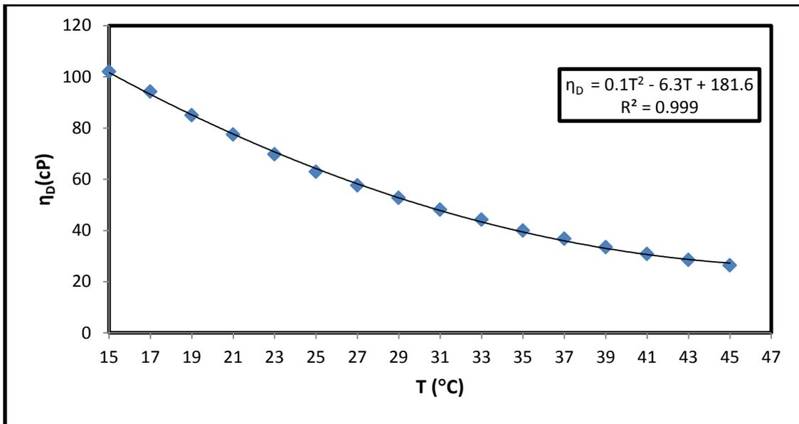
**Fig.(B.4):** Dynamic viscosity versus temperatures of Meithalun sample 2010 crop
