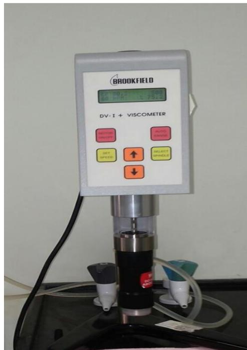
**Fig.(3.4):** DV-I viscometer
