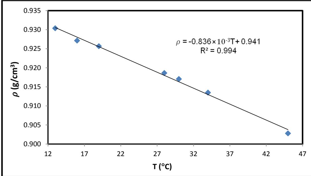
Fig. (A.5): The measured density for Allar sample from 2012 crop versus temperatures
