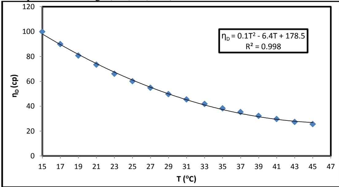
**Fig.(B.1):** Dynamic viscosity versus temperatures of Yatta sample 2012 crop
