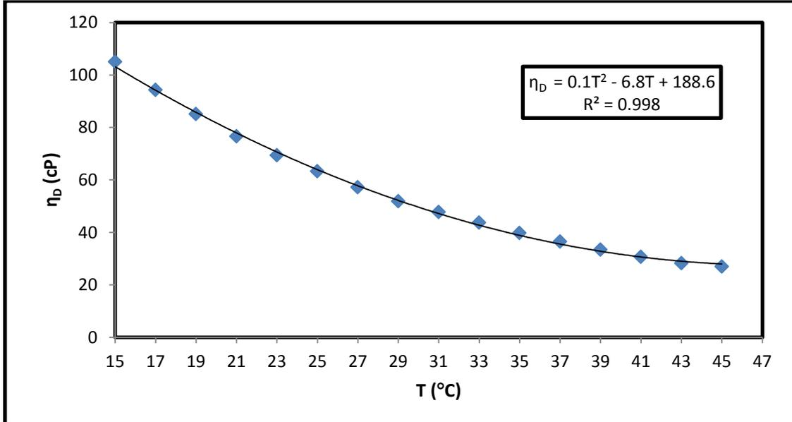
**Fig.(B.3):** Dynamic viscosity versus temperatures of Meithalun sample 2007 crop
