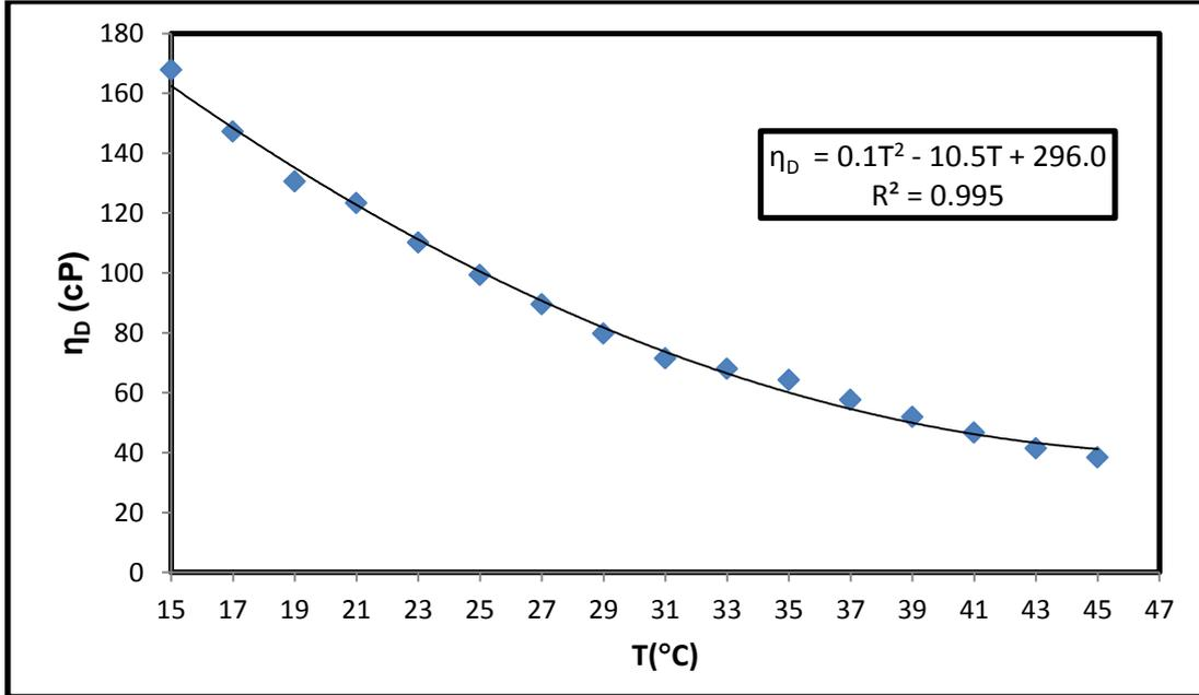
**Fig.(B.5):** Dynamic viscosity versus temperatures of Saida sample 1997 crop
