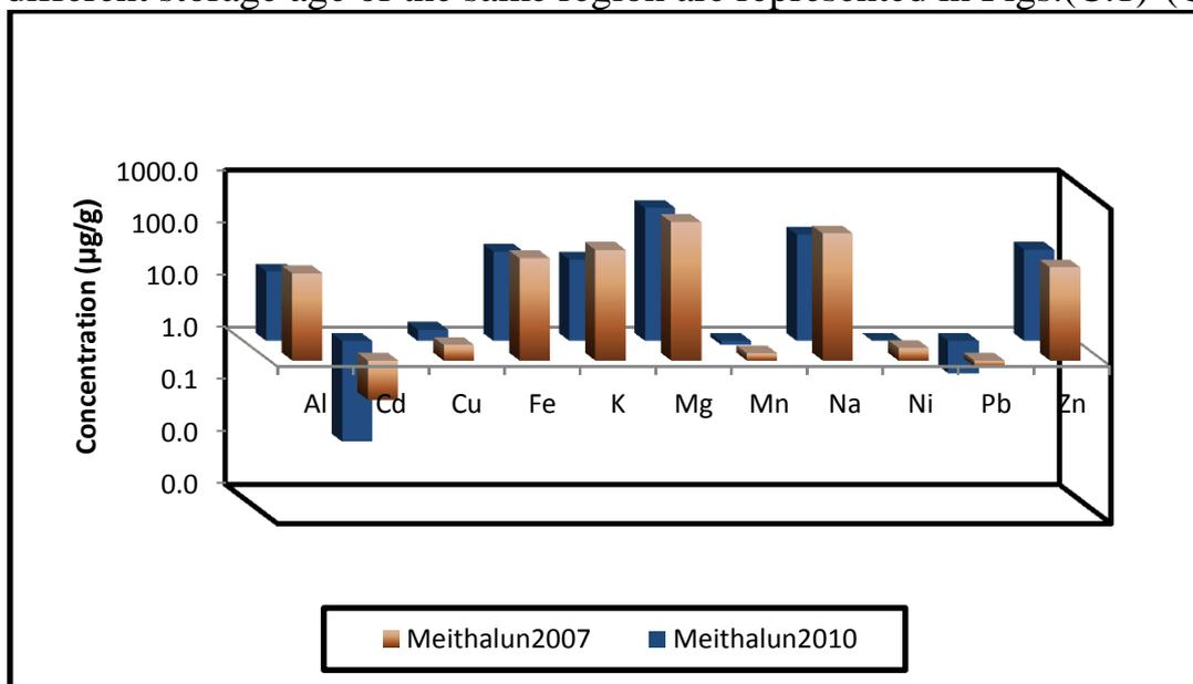
**Fig.(C.1):** The comparison between the levels of metals for two different storage age olive oil samples of same region(Meithalun)
