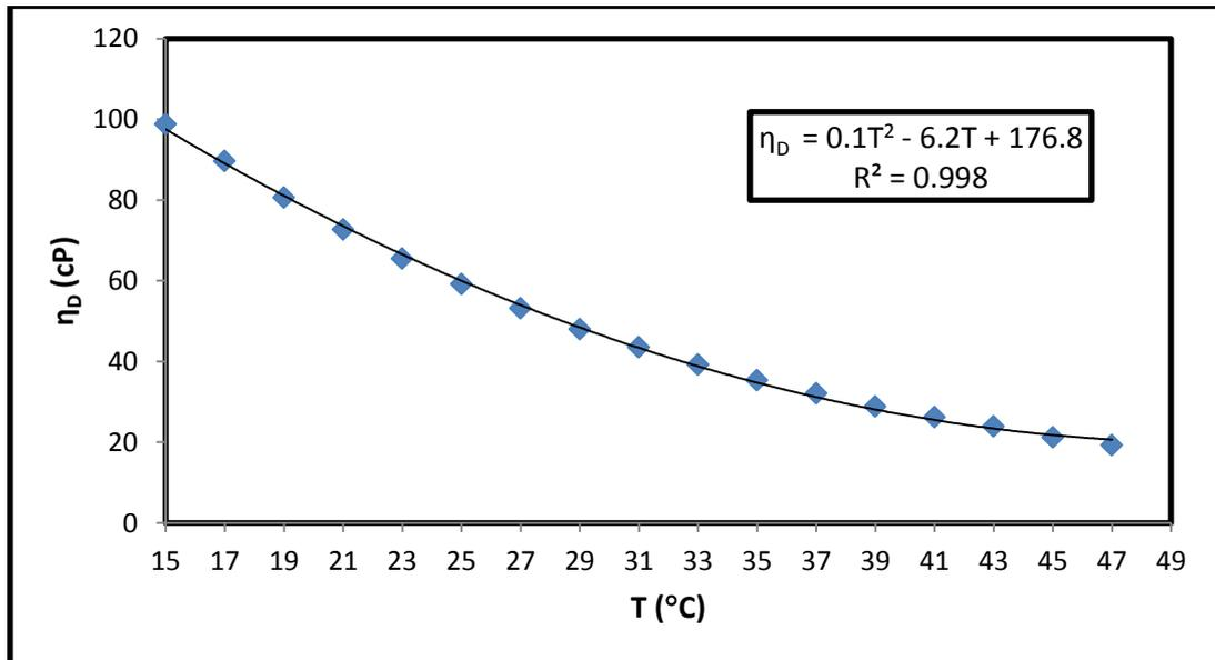
**Fig.(B.8):** Dynamic viscosity versus temperatures of Allar sample 1998 crop
