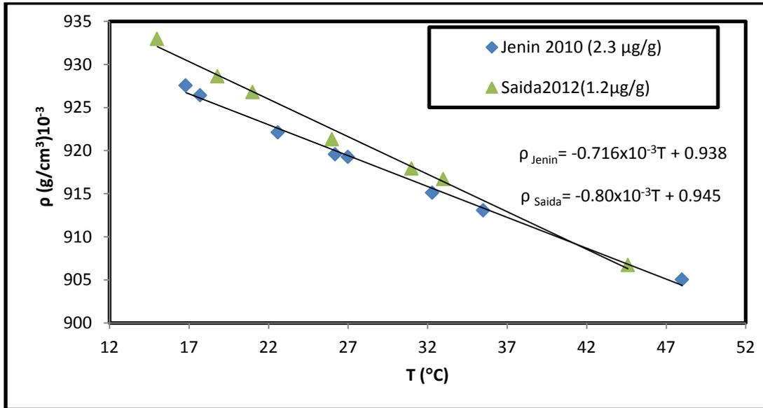
**Fig.(4.10):** The effect of two different concentrations of copper (Cu) on the density as function of temperature
