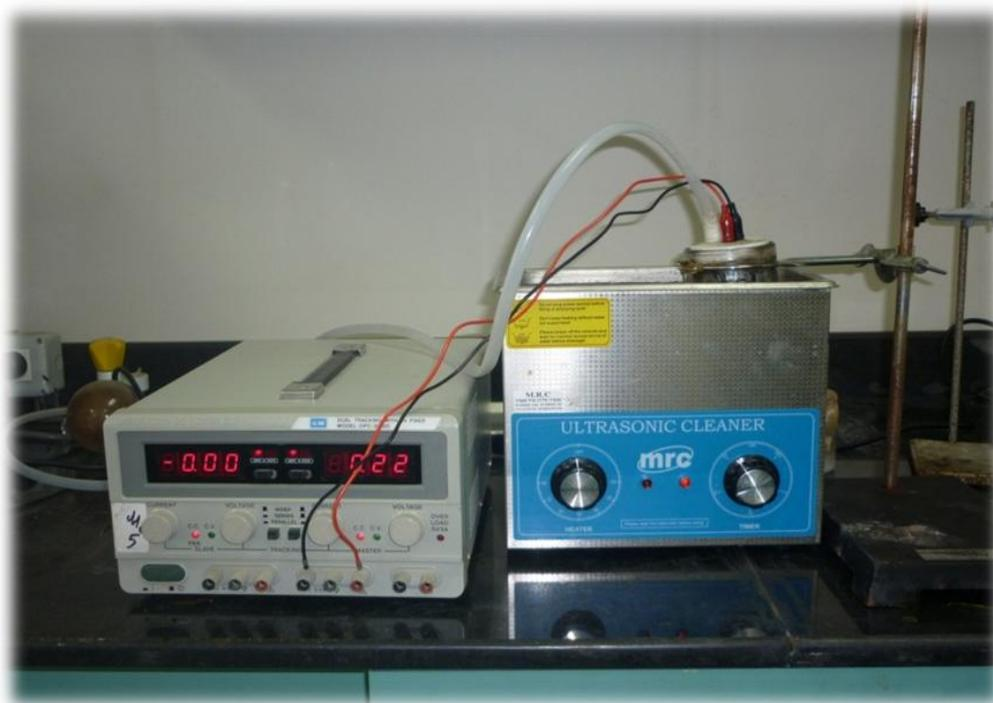
**Figure 3.1:** Photographic image for the setup that was used in the preparation of samples. Composed of three main parts: (I) electrolysis cell (Pd-anode, counter cathode and nitrogen inlet/outlet system), (II) power supply for current generation and (III) ultrasonic shaking system.
