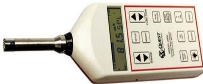
**Fig. 3.4** Sound level meter model 2900
