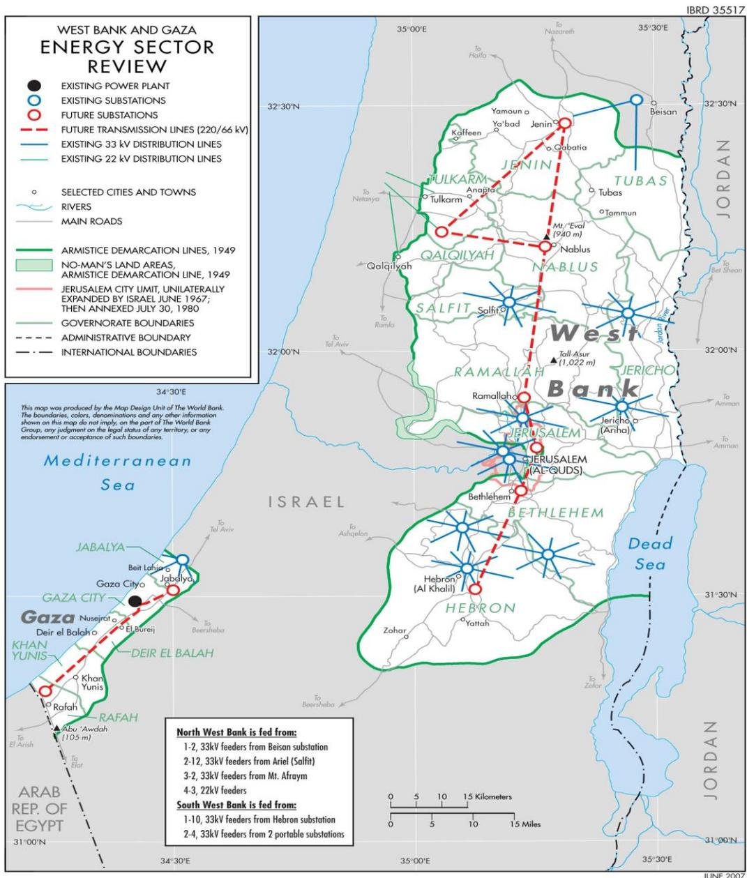
**Figure (1.1):** Electricity Supply System in West Bank and Gaza [2]
