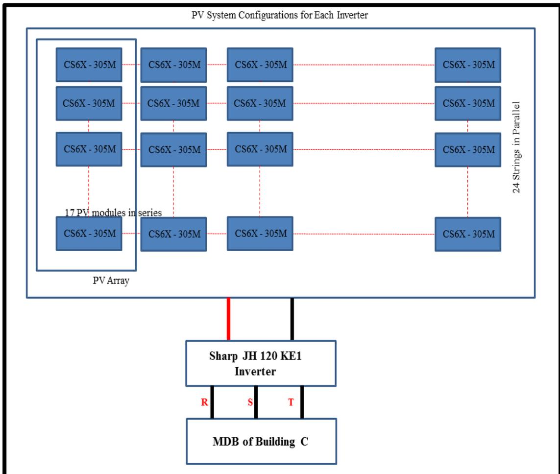
**Figure (4.6):** Building (C) PV System Schematic
