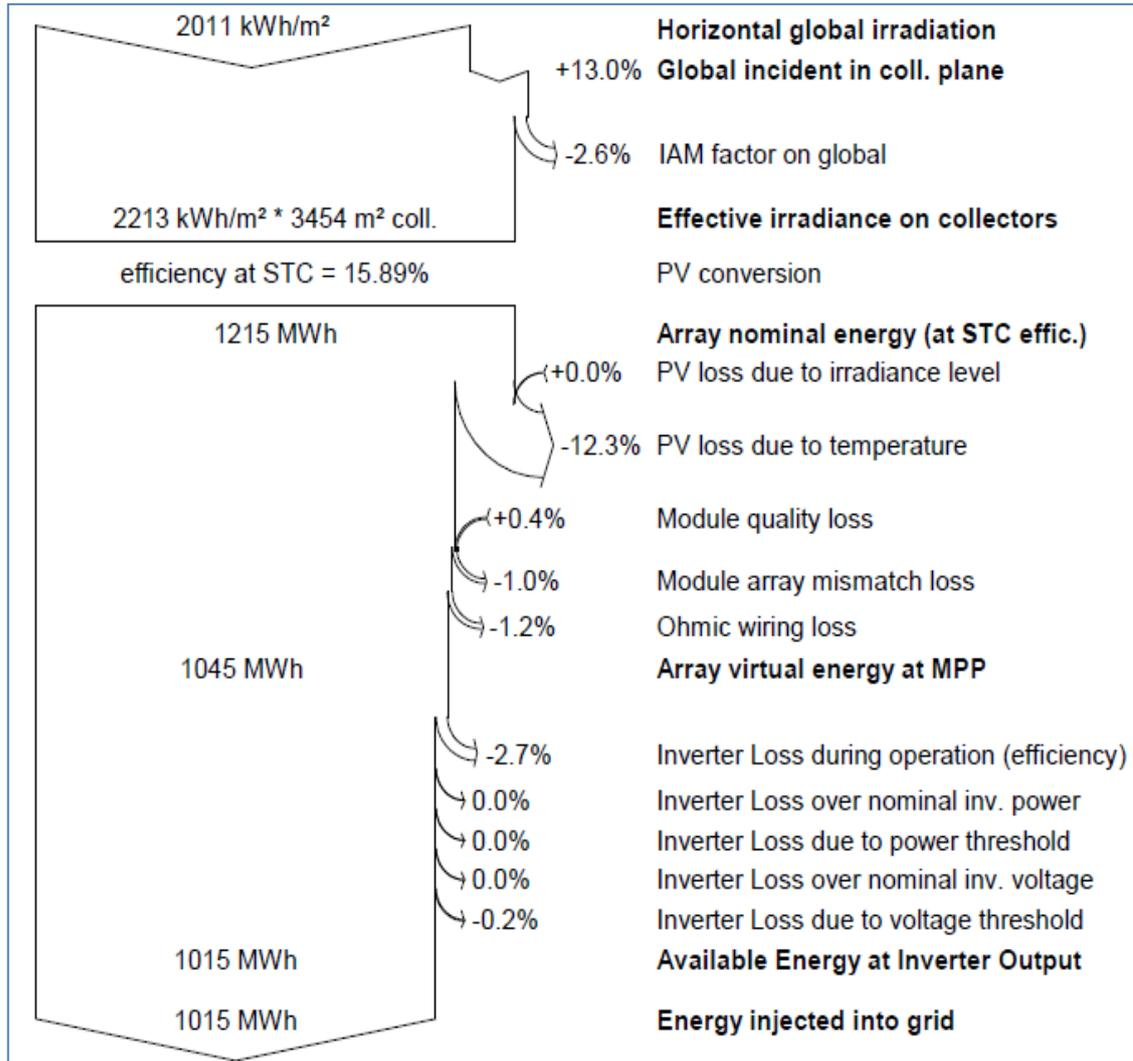
**Figure (4.8):** Building (A) PV system losses breakdown.
