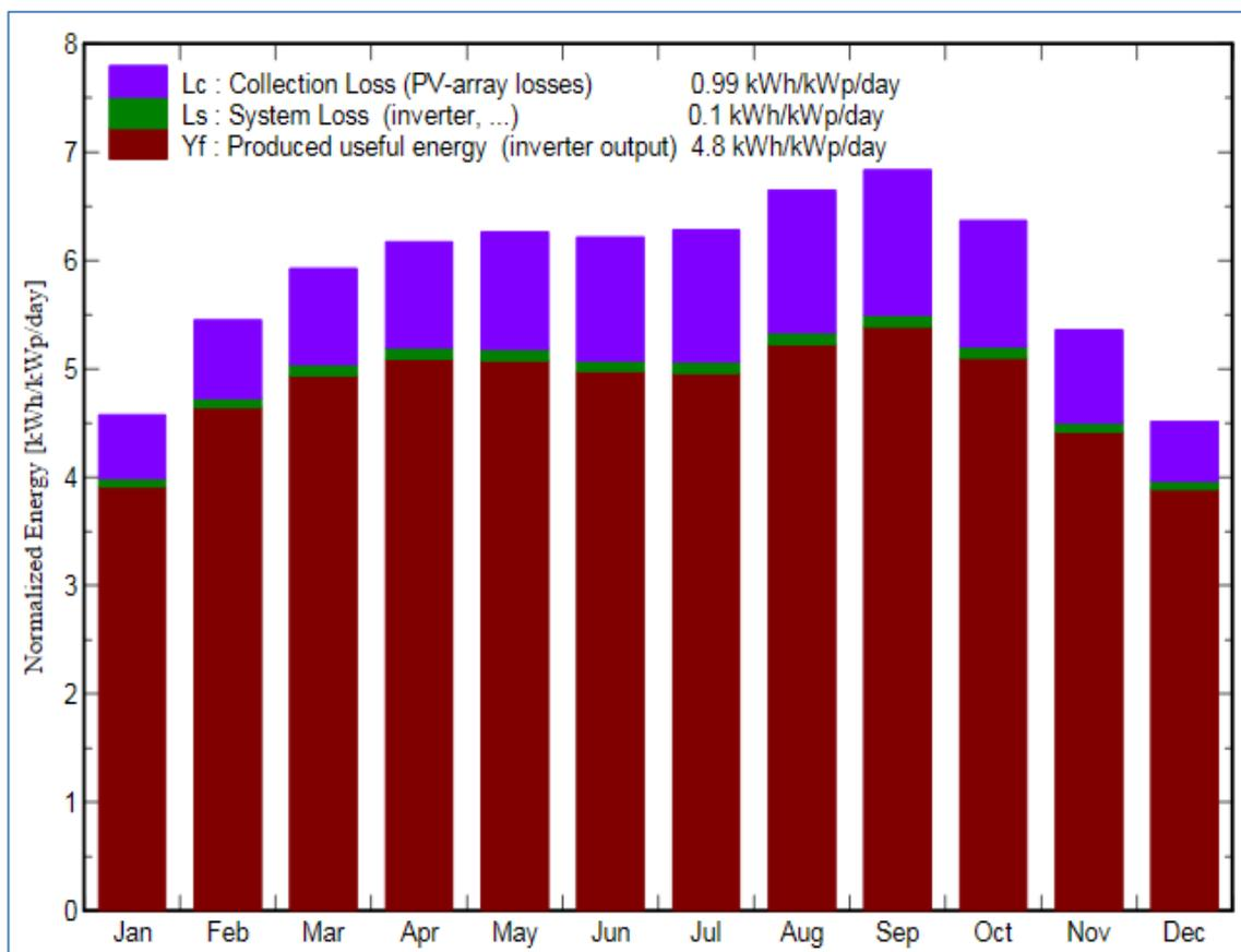
**Figure (4.9):** Normalized productions for building (B) (per installed kWp)
