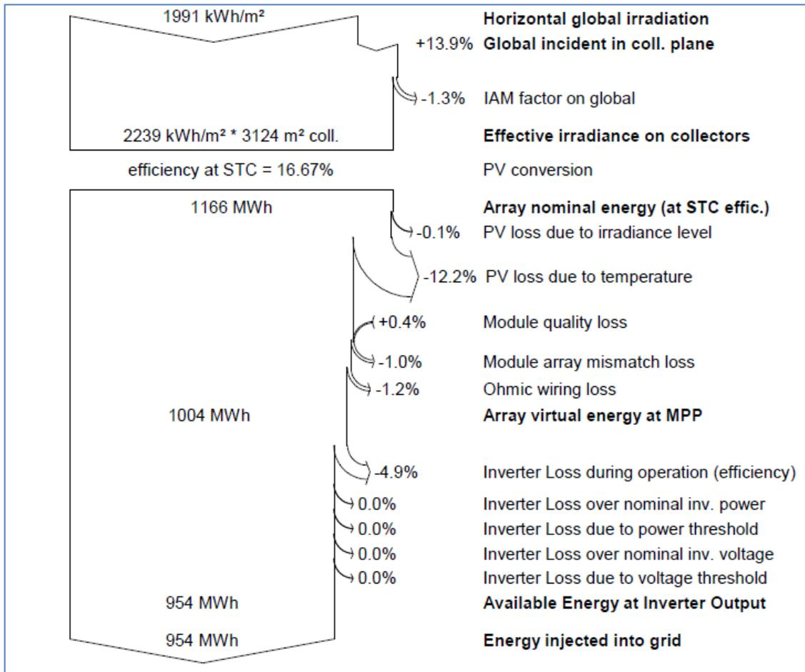
**Figure (4.12): Building (C) PV system losses breakdown.**
