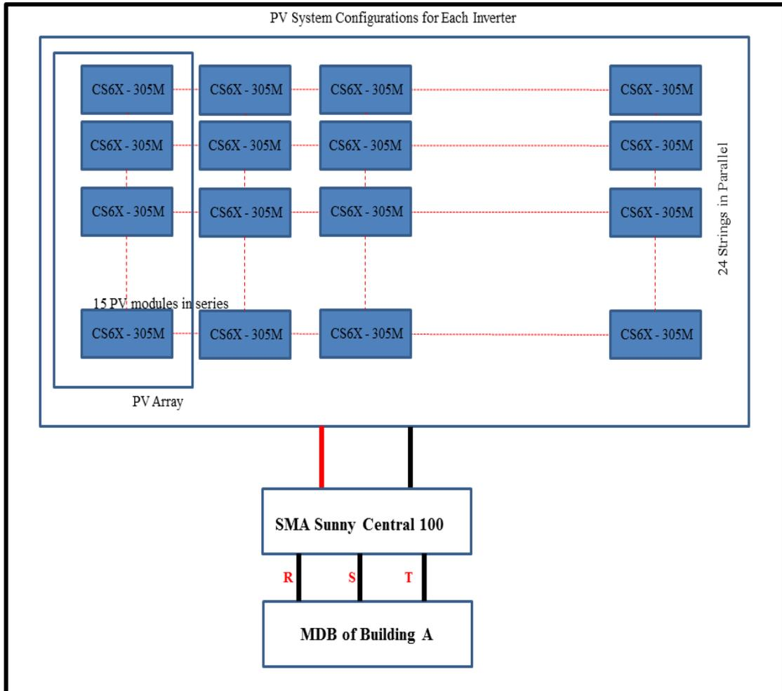
**Figure (4.4):** Building (A) PV System Schematic.
