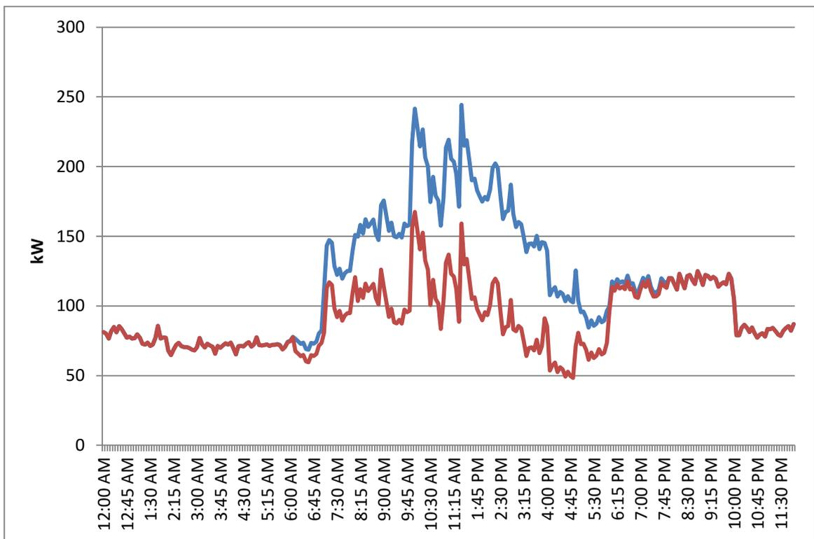
**Figure (5.13):** Daily Load Curve of Building (B) before and after PV Installation.
