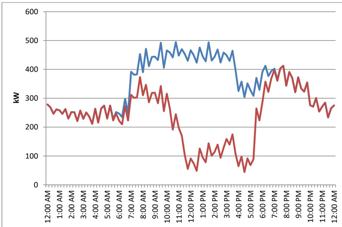
**Figure (5.15):** Daily Load Curve of Building (C) before and after PV Installation.
