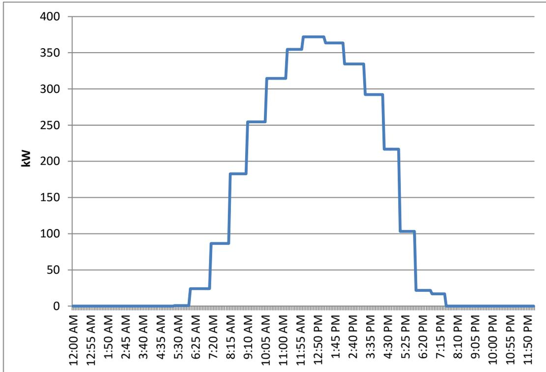
**Figure (5.9):** Building (C) PV System Output.
