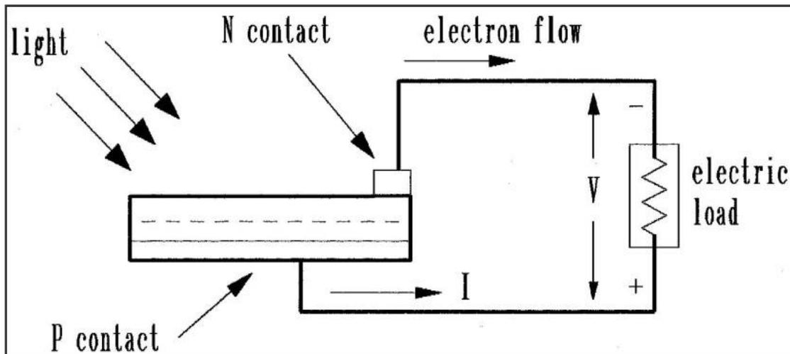
**Figure 2.2:** Photovoltaic effect converts the photon energy into voltage across the p-n junction. [6]
