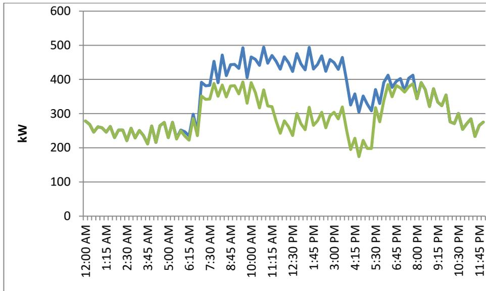
**Figure (5.16):** Proposed Daily Load Curve for Building (C) Using EMS.
