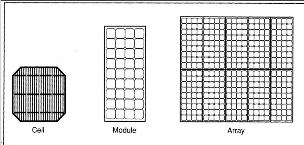
**Figure 2.4:** Cell, module, and array that form the solar system. [6]
