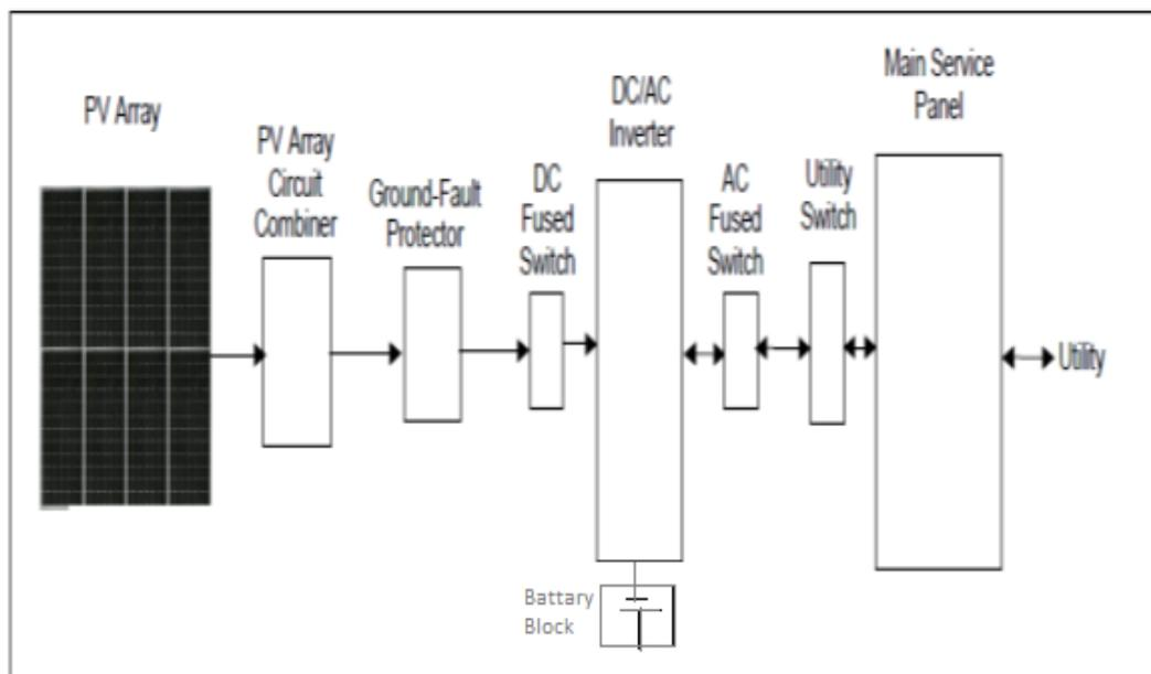
**Figure (2.1):** General Block Diagram of PV System. [7]
