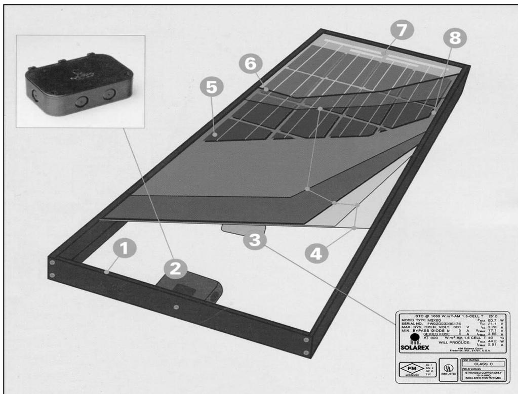
**Figure 2.5:** The module construction, consists of: (1) holding frame, (2) Weatherproof junction box, (3) The rating paper, (4) Transient material to protect from weathers and accident, (5) The PV cell, (6) High transmissivity glass, (7) Busses, (8) clearance. [6]
