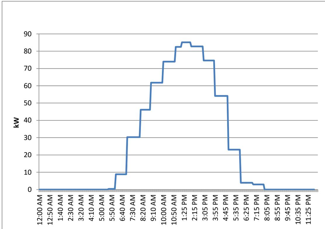
**Figure (5.6):** Building (B) PV System Output.
