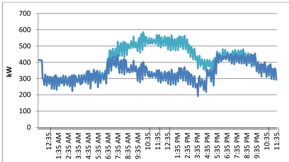
**Figure (5.12):** Proposed Daily Load Curve for Building (A) Using EMS.
