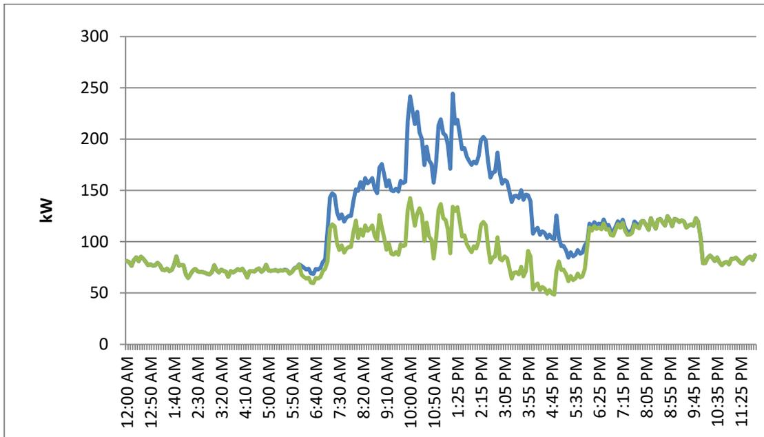
**Figure (5.14):** Proposed Daily Load Curve for Building (B) Using EMS.
