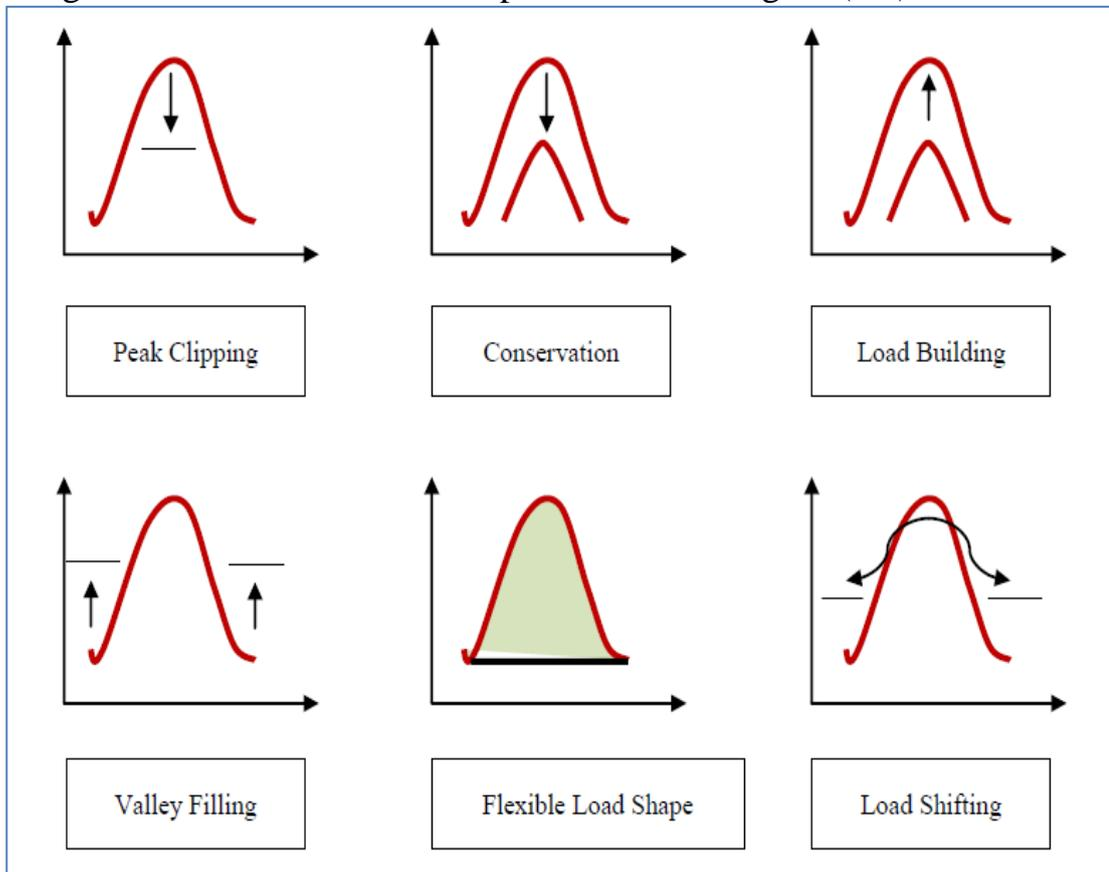
**Figure (3.2):** Load Shaping Techniques. [14]
