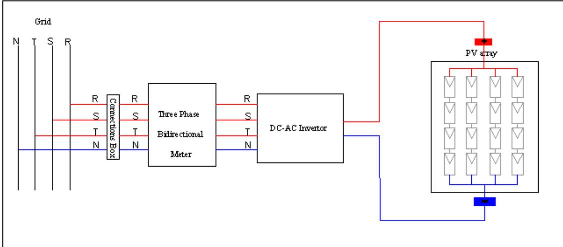
**Figure 2.7:** ON-grid PV system block diagram.
