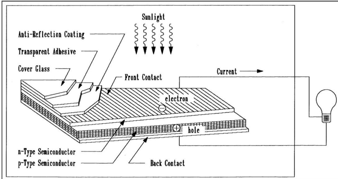
**Figure 2.3:** The PV construction with the addition of the mechanical developments. [6]
