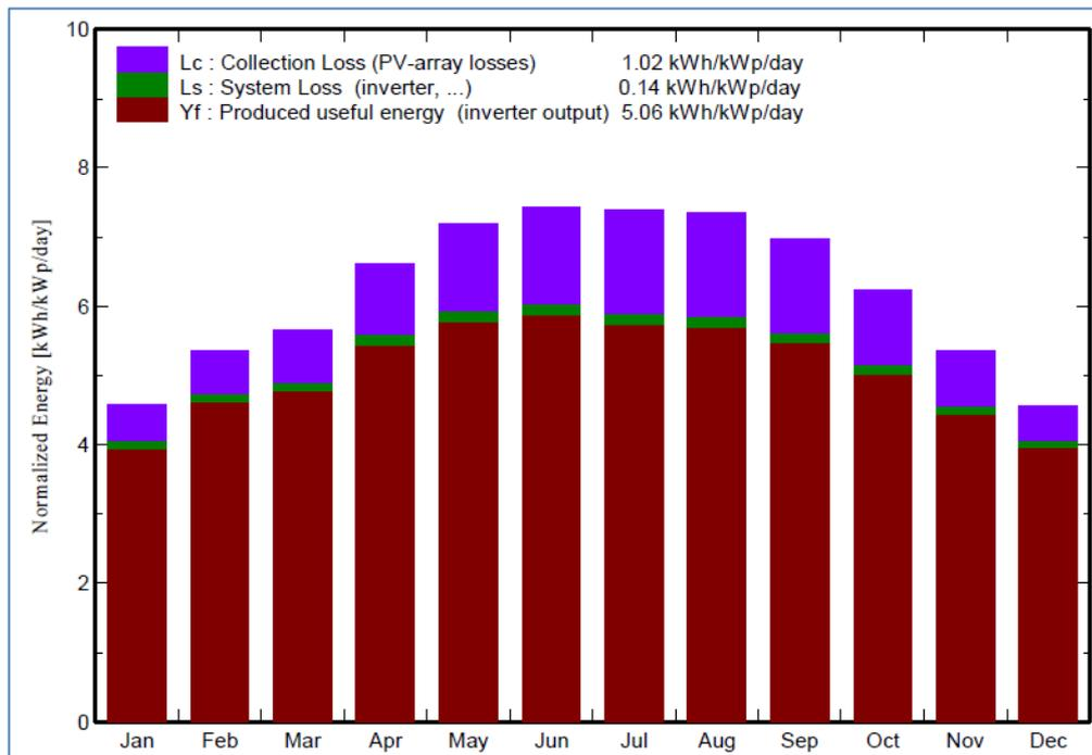
**Figure (4.7):** Normalized productions for building (A) (per installed kWp)
