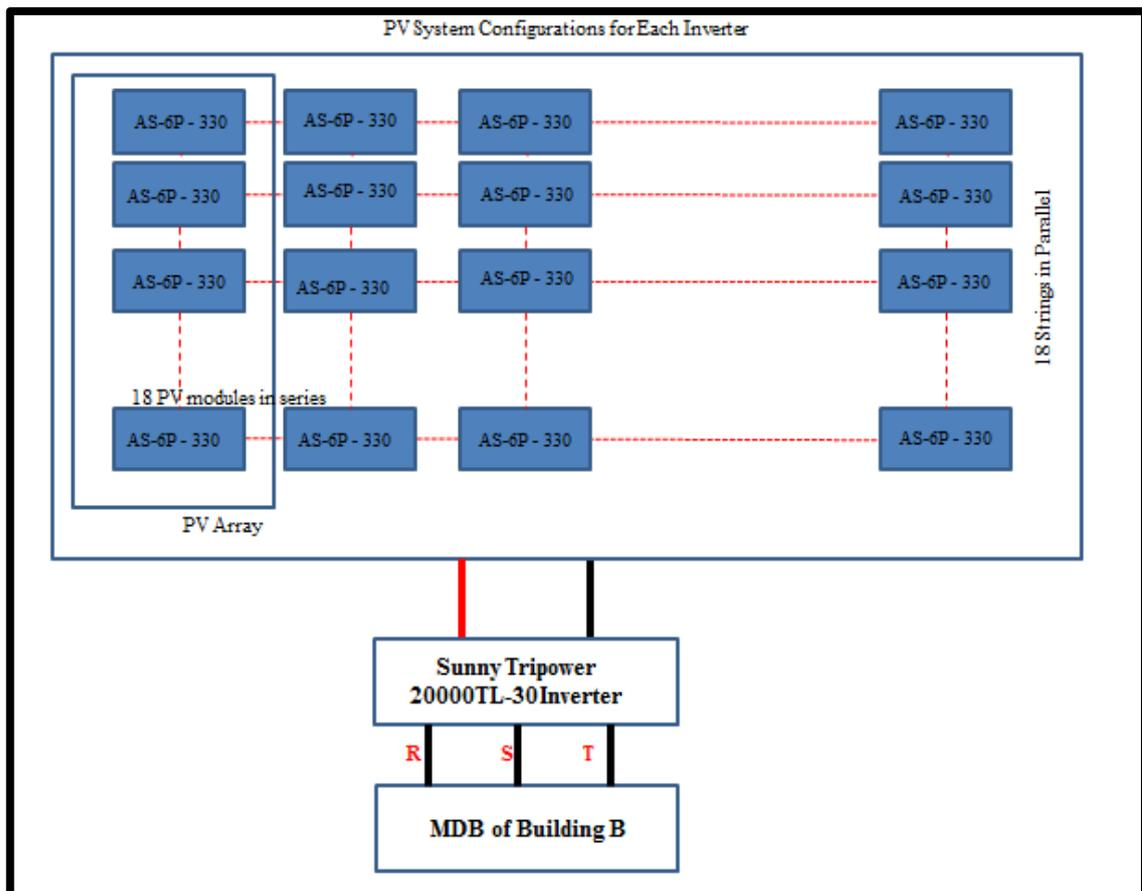
**Figure (4.5):** Building (B) PV System Schematic
