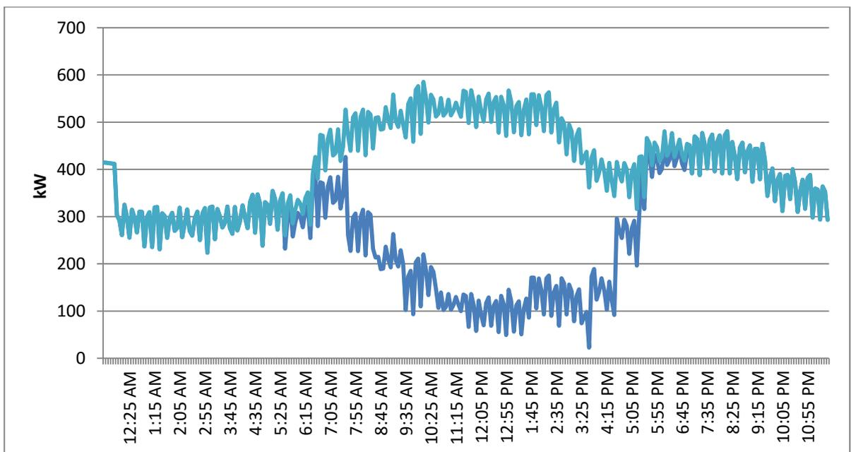
**Figure (5.11):** Daily Load Curve of Building (A) before and after PV Installation.
