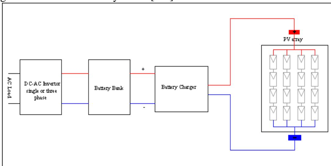
**Figure 2.6:** OFF-grid PV system block diagram.
