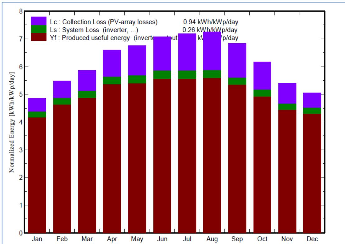
**Figure (4.11):** Normalized productions for building (C) (per installed kWp)
