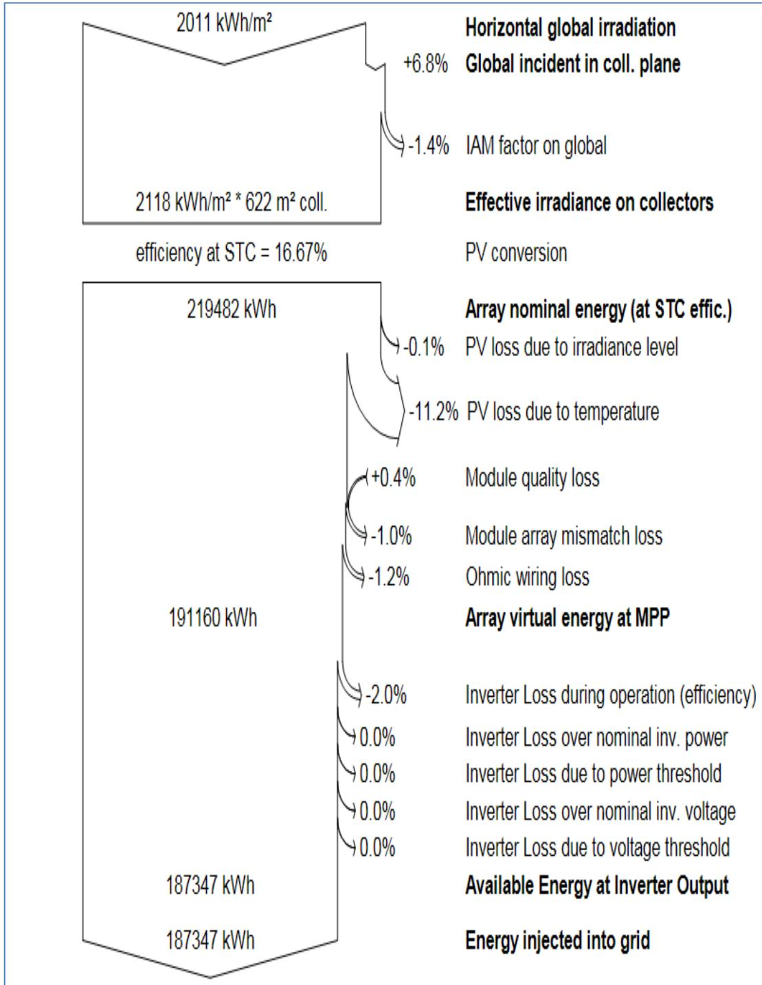
**Figure (4.10):** Building (B) PV system losses breakdown.
